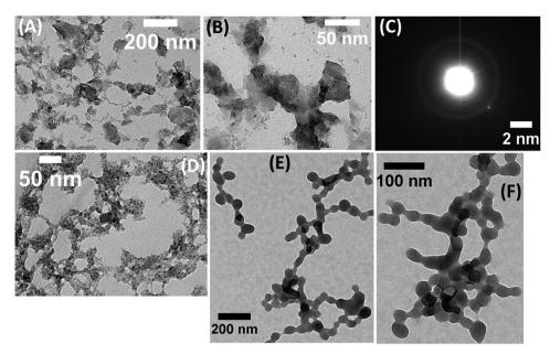
Fig. 3 Transmission electron microscopy (TEM) images of (A) and (B) PEI exfoliated q-C<sub>3</sub>N<sub>4</sub> nanosheets (PEI-q-C<sub>3</sub>N<sub>4</sub> NSs); (D)-(F) unmodified calcium alginate beads (Ca-Alg beads); (E) and (F) PEI-g-C<sub>3</sub>N<sub>4</sub> NSs@Ca-Alg beads; high-resolution transmission electron microscopy (HR-TEM) images of (C) the selected area electron diffraction (SAED) pattern for PEI-g-C<sub>3</sub>N<sub>4</sub> NSs
