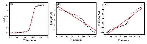
Fig. 5 (A) Thomas model breakthrough curve, (B) linear plot of the Thomas model and (C) linear plot of the Yoon-Nelson model.
