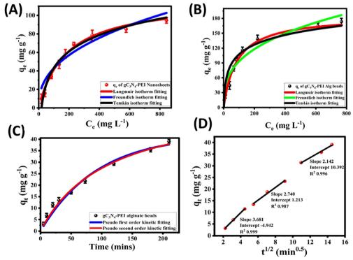
Fig. 4 (A) and (B) Non-linear fitting of the Langmuir (red curve), Freundlich (blue curve) and Temkin isotherms (black curve) for  $PEI-g-C_3N_4$ -NSs and calcium alginate beads (Ca-Alg beads) functionalized with  $PEI-g-C_3N_4$  NSs; (C) and (D) calcium alginate beads (Ca-Alg beads) functionalized with  $PEI-g-C_3N_4$  NSs for (C) non-linear pseudo-first-order kinetics and the pseudo-second-order kinetic model for (D) linear plot for intraparticle diffusion.
