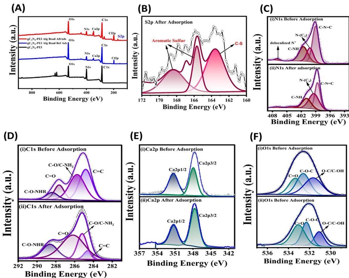
Fig. 1 (A) The total survey spectra of PEI exfoliated  $g\text{-C}_3\text{N}_4$  NSs, and also PEI exfoliated  $g\text{-C}_3\text{N}_4$ NSs@Cal–Alg beads before and after adsorption of DBT; (B)–(F) high-resolution deconvoluted spectra before and after adsorption of the DBT spectra for sulphur (B), nitrogen (N 1S) (C), carbon spectra C 1S (D), calcium (Ca 2p) spectra (E), and oxygen (O 1S) spectra (F).
