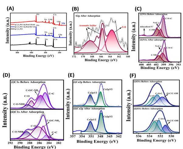
Fig. 1 (A) The total survey spectra of PEI exfoliated  $g-C_3N_4$  NSs, and also PEI exfoliated  $g-C_3N_4$ NSs@Cal-Alg beads before and after adsorption of DBT; (B)-(F) high-resolution deconvoluted spectra before and after adsorption of the DBT spectra for sulphur (B), nitrogen (N 1S) (C), carbon spectra C 1S (D), calcium (Ca 2p) spectra (E), and oxygen (O 1S) spectra (F).
