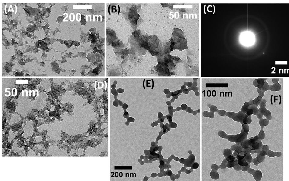
Fig. 3 Transmission electron microscopy (TEM) images of (A) and (B) PEI exfoliated  $g\text{-C}_3\text{N}_4$  nanosheets (PEI- $g\text{-C}_3\text{N}_4$  NSs); (D)–(F) unmodified calcium alginate beads (Ca-Alg beads); (E) and (F) PEI- $g\text{-C}_3\text{N}_4$  NSs@Ca-Alg beads; high-resolution transmission electron microscopy (HR-TEM) images of (C) the selected area electron diffraction (SAED) pattern for PEI- $g\text{-C}_3\text{N}_4$  NSs.
