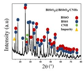
Fig. 2 XRD pattern of B@B/CNH nanocomposite.
