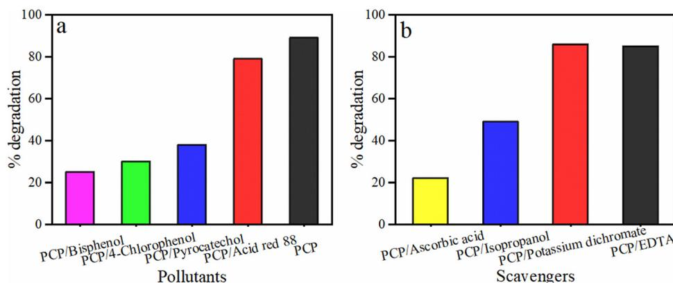
**Fig. 8** Effect of (a) different pollutants and (b) scavengers on the degradation efficiency of 5-CP by B@B/CNH nanocomposite.
