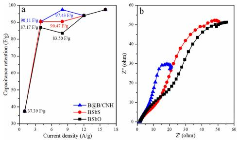
Fig. 10 Electrochemical study (a) graph of current density vs. capacitance retention for BSbO, BSbS, and B@B/CNH (b) EIS graphs with circuit for BSbO, BSbS, and B@B/CNH
