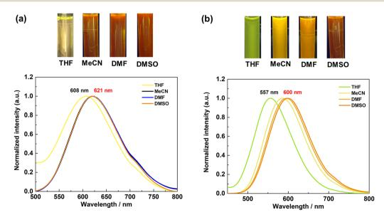
Fig. 1 Photographs (under UV irradiation at 365 nm) and normalized emission spectra ( $\lambda_{ex} = 420$  nm) for MTPA (a) and BTPA (b) in various solvents.
