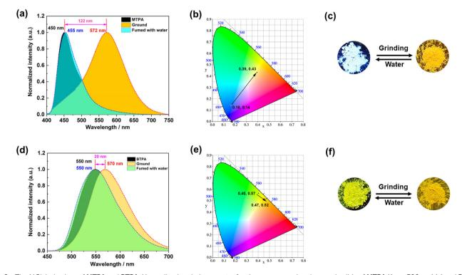
Fig. 2 The MCL behaviors of MTPA and BTPA. Normalized emission spectra for the as-prepared and ground solids of MTPA ( $\lambda_{ex}$  = 380 nm) (a) and BTPA ( $\lambda_{ex}$  = 420 nm) (d); the CIE-1931 chromaticity diagrams for the as-prepared and ground solids of MTPA (b) and BTPA (e); optical images in different solids for MTPA (c) and BTPA (f) under UV irradiation (365 nm).
