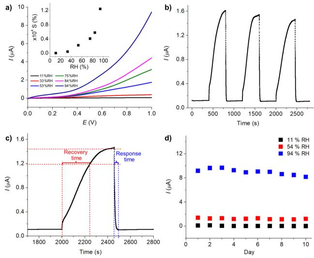
Fig. 6 (a) Current–voltage characteristics of the Cl-CuPc/PVP sensor across varying relative humidity (%RH) levels. The inset shows the plot of the humidity response (S) as a function of %RH. (b) Reproducibility of the Cl-CuPc/PVP sensor over three cycles at 11%RH and 94%RH. (c) Response and recovery time under fast change of %RH values between 11%RH and 94% RH. (d) Stability of the sensor over 10 days of storage at room temperature.
