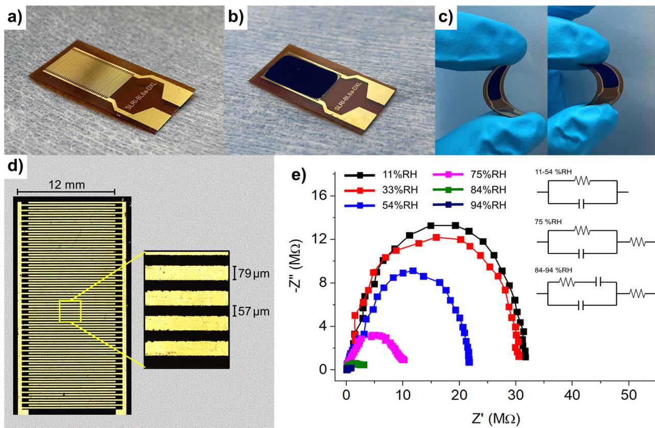
**Fig. 5** (a) A bare Au/Cr interdigitated electrode (Au/Cr-IDE). (b) Optical microscope image of the Au/Cr-IDE. (b) Cl-CuPc/PVP deposited on the Au/Cr-IDE. (c) Demonstration of the substrate's flexibility. (e) EIS spectra of Cl-CuPc/PVP/Au/Cr-IDE at different %RH.
