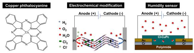
Scheme 1 (Left) Chemical structure of copper phthalocyanine (CuPc). (middle) Halide-mediated electrochemical modifications of CuPc. (right) Application of the electrochemically modified CuPc in a humidity sensor.
