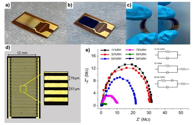
Fig. 5 (a) A bare Au/Cr interdigitated electrode (Au/Cr-IDE). (b) Optical microscope image of the Au/Cr-IDE. (b) Cl-CuPc/PVP deposited on the Au/Cr-IDE. (c) Demonstration of the substrate's flexibility. (e) EIS spectra of Cl-CuPc/PVP/Au/Cr-IDE at different %RH.
