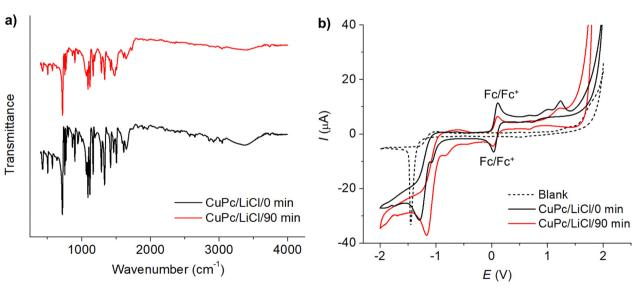
Fig. 4 (a) FTIR spectra of CuPc before modification (black line) and after modification (red line) in 0.50 M LiCl for 90 minutes. (b) Cyclic voltammograms of 1.0 mM CuPc before modification (black line) and after modification (red line) in the presence of 1.0 mM ferrocene and 0.10 M TBAPF<sub>6</sub> in acetonitrile at a scan rate of 50 mV s<sup>-1</sup>.
