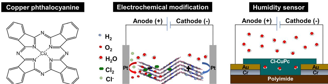
**Scheme 1** (Left) Chemical structure of copper phthalocyanine (CuPc). (middle) Halide-mediated electrochemical modifications of CuPc. (right) Application of the electrochemically modified CuPc in a humidity sensor.
