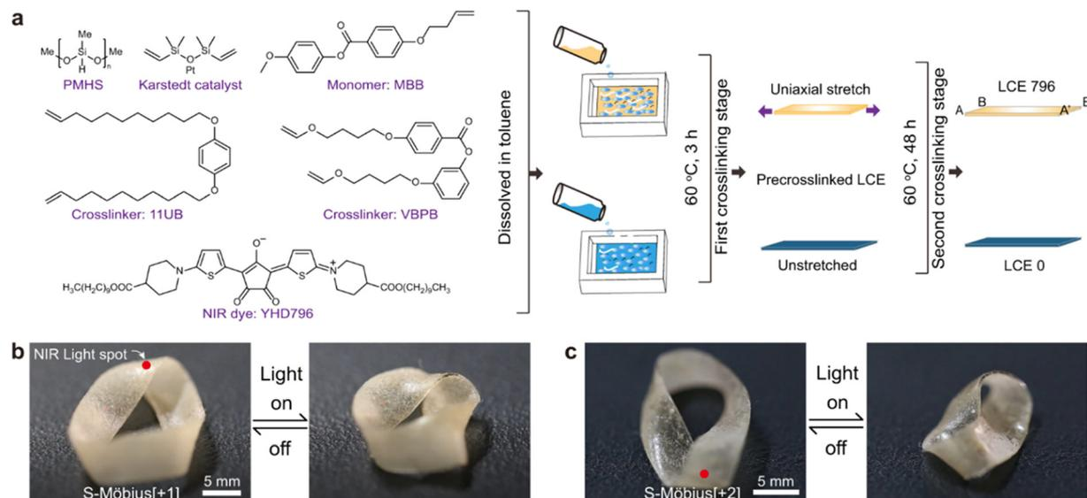
**Fig. 13** Dual-layer polysiloxane-based liquid crystal soft actuators. (a) Schematic illustration of the chemical components of this LCE system and the preparation procedure of LCE796 (orange part) and LCE0 (dark blue part) ribbons. Photographs of the single-layered (b) S-Möbius[+1] and (c) S-Möbius[+2] actuators upon application of a photothermal stimulus (scale bars: 5 mm) Reproduced with permission from ref. 100. Copyright 2021, Springer Nature.
