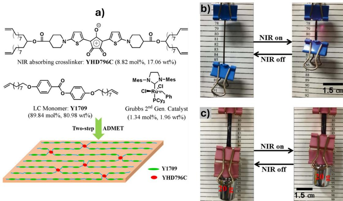
**Fig. 12** (a) Chemical composition of the LCE material; (b) photo image of an LCE ribbon before and after NIR (808 nm) irradiation; and (c) photo image of an LCE film (4.3 mg) lifting up a load (ca. 24.44 g) under NIR irradiation. Reproduced with permission from ref. 99. Copyright 2017, the American Chemical Society.
