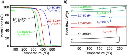
Fig. 4 (a) Thermal stability curves of the BCzPhs, recorded under a nitrogen gas atmosphere at a heating rate of 20 °C min<sup>-1</sup>. (b) DSC traces of the heating and cooling cycles of **BCzPhs** under nitrogen gas atmosphere at a scan rate of 10 °C min<sup>-1</sup>.
