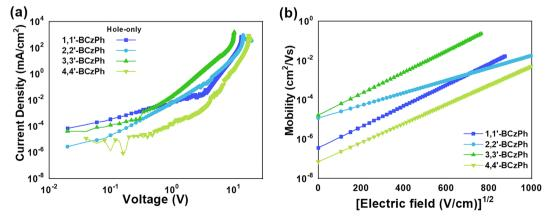
Fig. 7 (a) Current density-voltage (J-V) curves of the hole-only devices and (b) comparative field dependence mobility of **BCzPh**-based compounds.
