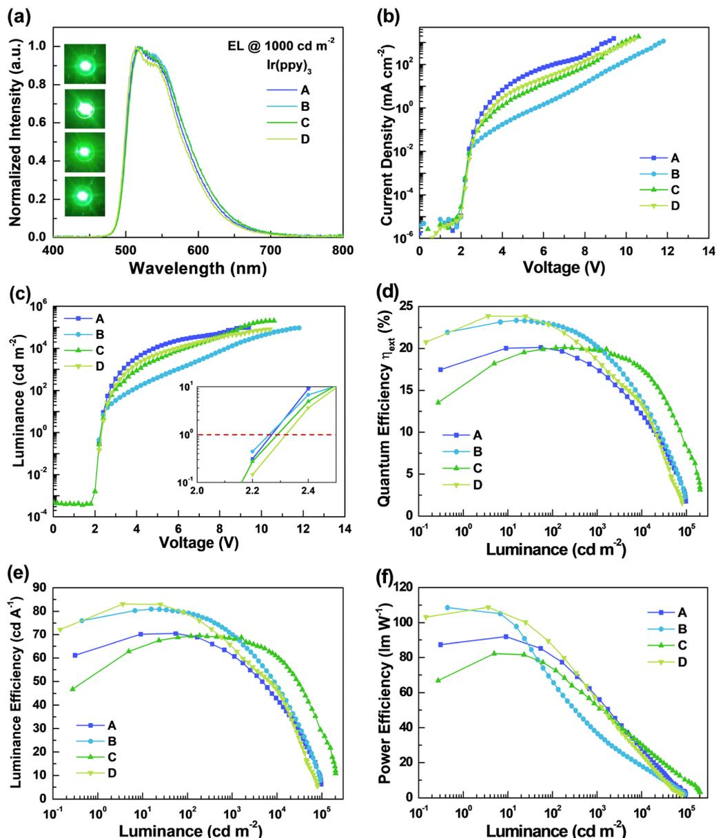
Fig. 10 (a) Normalized EL spectra at a luminance of  $1000 \text{ cd m}^{-2}$ ; (b) current density–voltage ( $J$ – $V$ ) characteristics; (c) luminance–voltage ( $L$ – $V$ ) characteristics; (d) external quantum efficiency (EQE) vs. luminance plot; (e) luminance efficiency vs. luminance plot; (f) power efficiency vs. luminance plot for devices A, B, C, and D. (The blended ratio of the co-host is **BCzPh**:B3PyMPPM = 1:1.)
