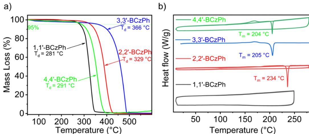
Fig. 4 (a) Thermal stability curves of the **BCzPhs**, recorded under a nitrogen gas atmosphere at a heating rate of  $20\text{ }^{\circ}\text{C min}^{-1}$ . (b) DSC traces of the heating and cooling cycles of **BCzPhs** under nitrogen gas atmosphere at a scan rate of  $10\text{ }^{\circ}\text{C min}^{-1}$ .
