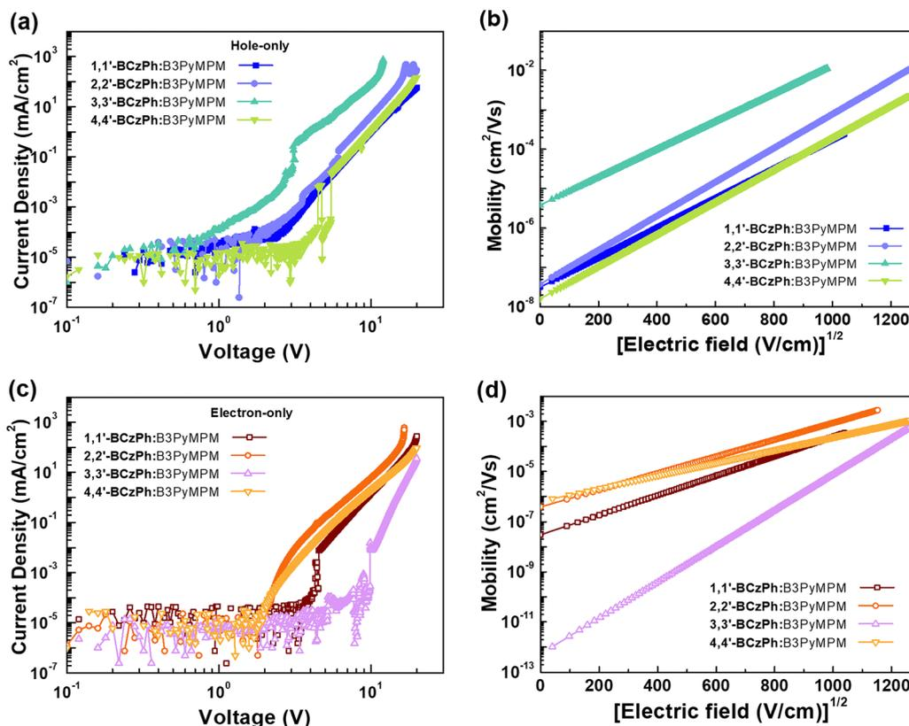
Fig. 8 (a) Current density–voltage ( $J$ – $V$ ) curves of the hole-only devices; (b) comparative field dependence hole mobility of **BCzPh**:B3PyMPM-based samples; (c) current density–voltage ( $J$ – $V$ ) curves of the electron-only devices; (d) comparative field dependence electron mobility of **BCzPh**:B3PyMPM-based samples.
