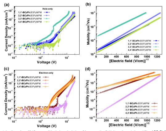
Fig. 8 (a) Current density-voltage (J-V) curves of the hole-only devices; (b) comparative field dependence hole mobility of **BCzPh**:B3PyMPM-based samples; (c) current density-voltage (J-V) curves of the electron-only devices; (d) comparative field dependence electron mobility of **BCzPh**:B3PyMPM-based samples.
