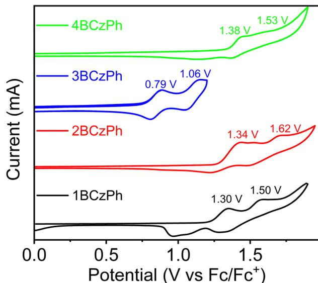
Fig. 3 Cyclic voltammograms of **BCzPhs** (1.0 mM) recorded in dichloromethane using **TBAPF<sub>6</sub>** (0.1 M) as the supporting electrolyte.
