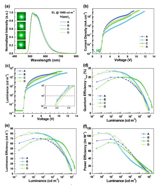
Fig. 10 (a) Normalized EL spectra at a luminance of 1000 cd m $^{-2}$ ; (b) current density-voltage (J-V) characteristics; (c) luminance-voltage (L-V) characteristics; (d) external quantum efficiency (EQE) vs. luminance plot; (e) luminance efficiency vs. luminance plot; (f) power efficiency vs. luminance plot for devices A, B, C, and D. (The blended ratio of the co-host is **BCzPh**: B3PyMPM = 1:1.)
