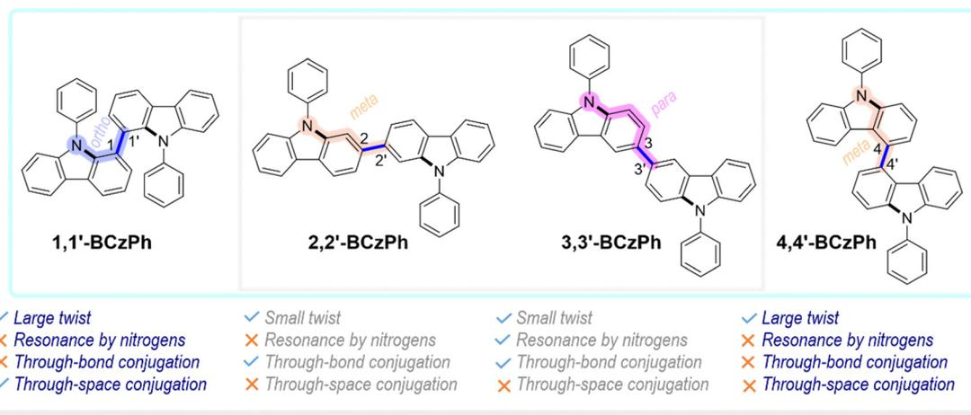
**Chart 1** Regioisomeric symmetric bicarbazole (**BCzPh**) emissive host materials investigated for PhOLED applications in this report and their molecular features. The *ortho*, *meta* and *para* relationships between the C–C and C–N bonds are highlighted.
