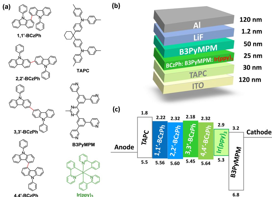
Fig. 9 (a) Schematic illustration of materials used in OLEDs; (b) schematic illustration of green phosphorescent OLED device structures with different host systems; (c) energy level alignment diagram of the used materials.
