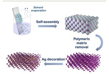
Scheme 1 Schematic of the co-assembly fabrication of Ag-WO<sub>3</sub>/TiO<sub>2</sub>
