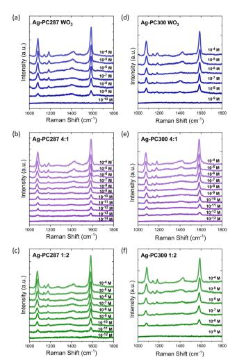
Fig. 6 SERS spectra of 4-MBA as a function of concentration ( $10^{-4}$ - $10^{-13}$  M) on (a) Ag-PC287 WO<sub>3</sub>, (b) Ag-PC287 4:1, (c) Ag-PC287 1:2, (d) Ag-PC300 WO<sub>3</sub>, (e) Ag-PC300 4:1 and (f) Ag-PC300 1:2 inverse opal substrates of variable macropore size and composition.
