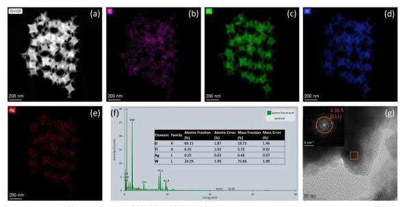
Fig. 2 (a) TEM image of Aq-PC287 4:1 film and the (b) Ti, (c) W, (d) O and (e) Ag elemental maps obtained from the corresponding (f) EDX spectrum (g) high-resolution TEM image and the corresponding FFT pattern for the squared area over a relatively isolated NP identifying the (111) planes of Ag (fcc) with 2.36 Å interplanar spacing.
