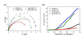
Fig. 7 Comparative (a) Nyquist and (b) Mott-Schottky plots for PC287 4:1 and TiO<sub>2</sub> substrates before and after Ag deposition at 500 Hz
