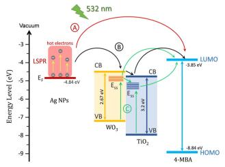
Fig. 8 Proposed charge transfer pathways in the Ag-WO<sub>3</sub>/TiO<sub>2</sub> system for 4-MBA SERS detection.
