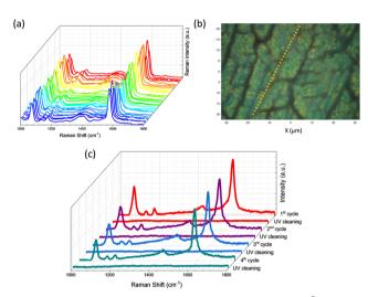
Fig. 10 (a) SERS spectra collected from 30 points for 10<sup>-5</sup> M 4-MBA detection on the Ag-PC287 4:1 substrate along the yellow line shown in the (b) image of the selected area. (c) SERS spectra of  $10^{-6}$  M 4-MBA on Ag-PC287 4:1 substrate for 4 cycles with intermediate UV-vis treatments.
