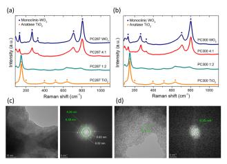
Fig. 3 Raman spectra for the (a) PC287 and (b) PC300 WO<sub>3</sub>/TiO<sub>2</sub> substrates at 532 nm. High resolution TEM images for (c) the plain PC287 WO<sub>3</sub> and (d) PC287 1:2 films and the corresponding FFT patterns for the whole TEM image in (c) and the squared area in (d).
