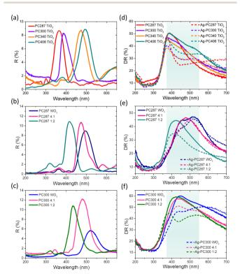
Fig. 4 (a)-(c) Specular reflectance R% spectra showing the Bragg reflection for the WO<sub>3</sub>/TiO<sub>2</sub> PC films. (d)-(f) Diffuse reflectance DR% spectra for the WO<sub>3</sub>/TiO<sub>2</sub> (solid lines) and Ag-WO<sub>3</sub>/TiO<sub>2</sub> (dashed lines) PC substrates. The cyan band delineates the spectral region of plasmonic Ag NP absorption on the metal oxide films
