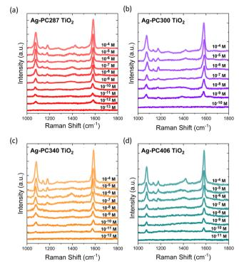
Fig. 5 SERS spectra of 4-MBA of variable concentrations ( $10^{-4}$ - $10^{-13}$  M) on Ag-TiO<sub>2</sub> (a) PC287, (b) PC300, (c) PC340 and (d) PC406 inverse opal substrates of different macropore diameter and PBG.
