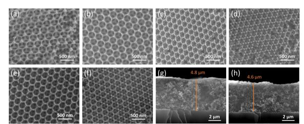
Fig. 1 Top-view SEM images for PC287 (a) WO<sub>3</sub>, (b) 4:1, (c) 1:2, (d) TiO<sub>2</sub> as well as (e) Ag-PC287 4:1, and (f) Ag-PC287 1:2 substrates. Cross-section SEM images for PC287 (g) 4:1 and (h) 1:2 films.
