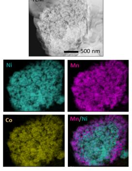
Fig. 6 TEM-EDS study of a Ni-rich core/Mn-rich shell particle.
