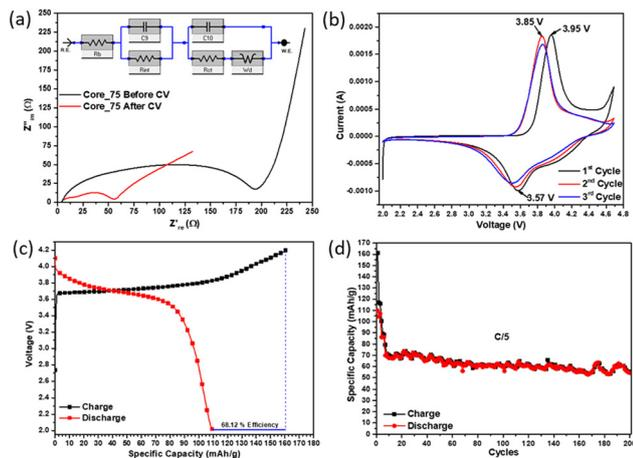
Fig. 10 Electrochemical analysis of the Core\_75 sample (a) before CV and after CV EIS spectra comparison. (b) CV analysis. (c) First formation cycle coulombic efficiency result. (d) GCD test result at 0.2C starting from the formation test.
