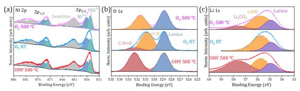
Fig. 9 In situ XPS spectra of (a) Ni 2p, (b) O 1s and (c) Li 1s core levels acquired under UHV at 500 °C, and under an O2 atmosphere at room temperature and 500 °C
