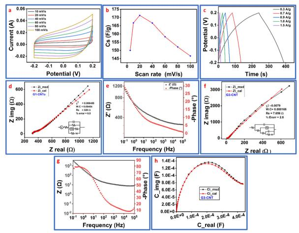
Fig. 8 Electrochemical properties; (a) CV at different scan rates for G3-CNT, (b) specific capacitance (F  $g^{-1}$ ) vs. different scan rates for G3-CNT, (c) GCD at different current densities for G3-CNT, (d) EIS Nyquist for G1-CNT<sub>0</sub>, (e) Bode plot of G1-CNT<sub>0</sub>, (f) Nyquist plot of G3-CNT and electronic circuit inset, (g) G3-CNT bode plot at high and low frequency regions, and (h) G3-CNT capacitance between imaginary and real values.
