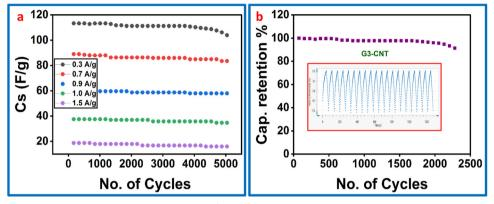
Performance evaluation of the G3-CNT hydrogel; (a) Cs (F  $q^{-1}$ ) after 5000-cycle operation and (b) capacitance retention % vs. number of cycles.
