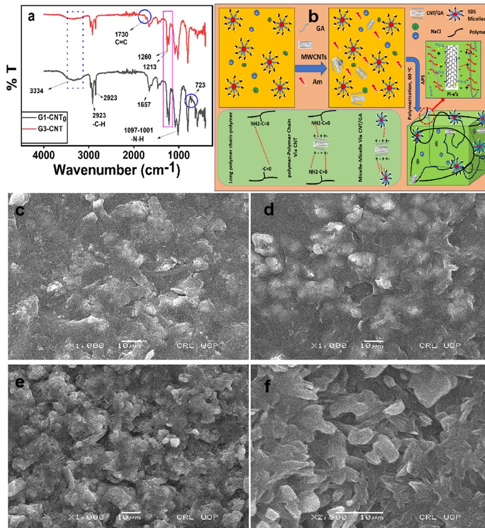
Fig. 1 (a) FT-IR spectra, (b) the existence of a possible interaction in the hydrogel network, and SEM images of (c) G1-CNT<sub>0</sub>, (d) G1-CNT, (e) G2-CNT, and (f) G3-CNT.
