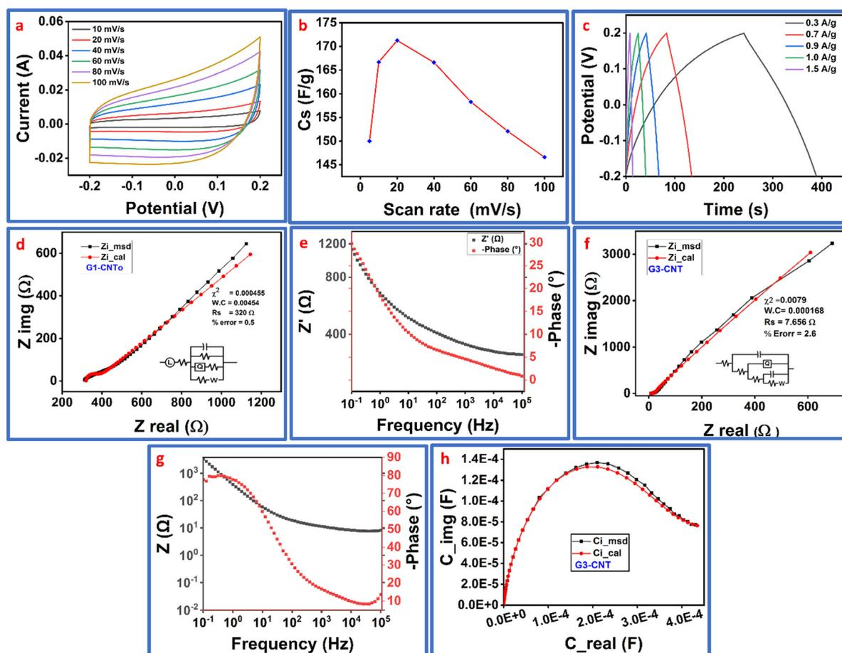
Fig. 8 Electrochemical properties; (a) CV at different scan rates for G3-CNT, (b) specific capacitance ( $\text{F g}^{-1}$ ) vs. different scan rates for G3-CNT, (c) GCD at different current densities for G3-CNT, (d) EIS Nyquist for G1-CNT<sub>0</sub>, (e) Bode plot of G1-CNT<sub>0</sub>, (f) Nyquist plot of G3-CNT and electronic circuit inset, (g) G3-CNT bode plot at high and low frequency regions, and (h) G3-CNT capacitance between imaginary and real values.
