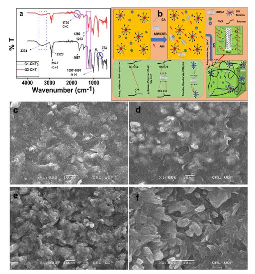
Fig. 1 (a) FT-IR spectra, (b) the existence of a possible interaction in the hydrogel network, and SEM images of (c) G1-CNT<sub>0</sub>, (d) G1-CNT, (e) G2-CNT, and (f) G3-CNT.
