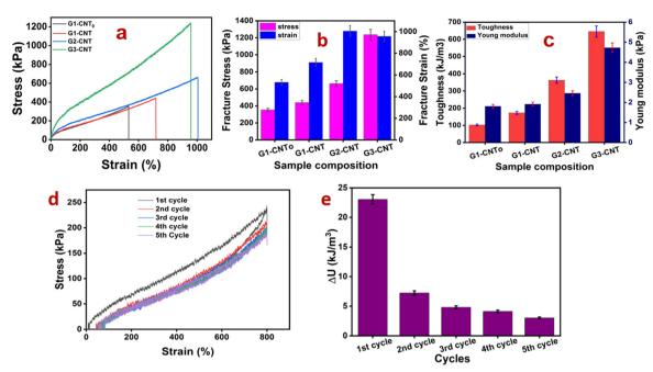
Fig. 2 Mechanical performance of the G3-CNT hydrogel: (a) tensile stress-strain test, (b) fracture stress and strain values, (c) toughness and Young's modulus, (d) cyclic tensile loading-unloading test without any rest time, and (e) dissipated energy in various cycles.
