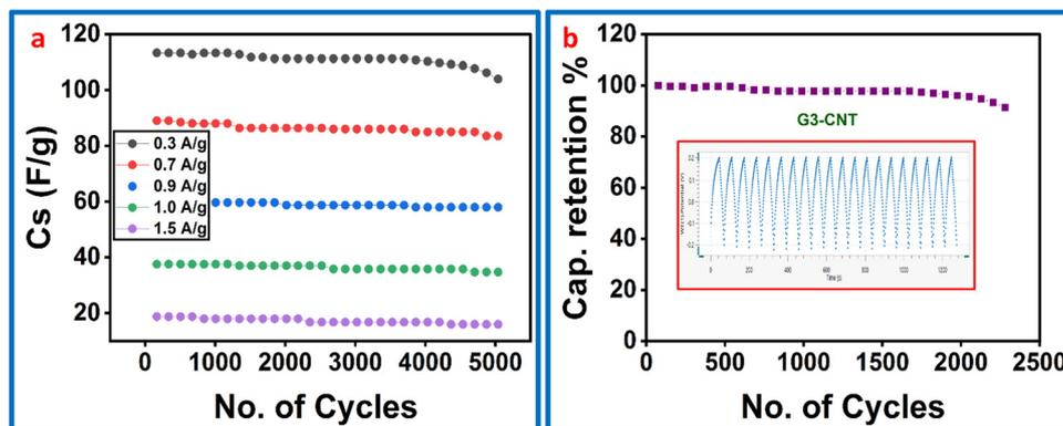
Fig. 9 Performance evaluation of the G3-CNT hydrogel; (a)  $C_s$  (F g<sup>-1</sup>) after 5000-cycle operation and (b) capacitance retention % vs. number of cycles.
