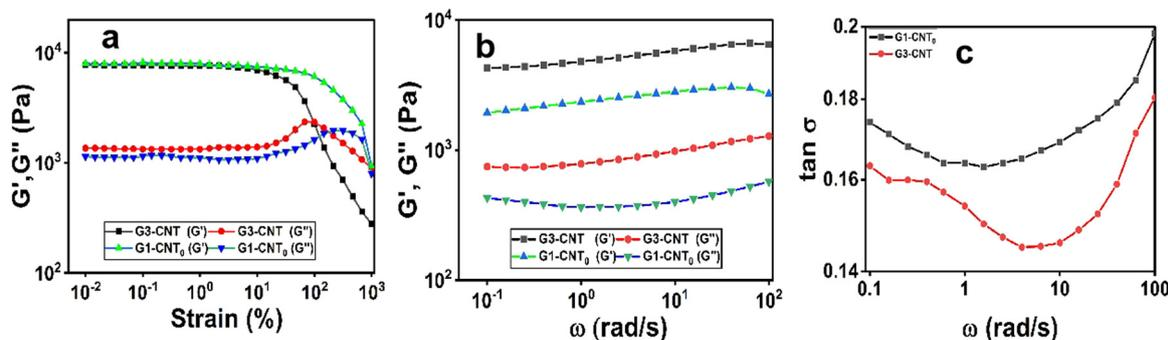
Fig. 3 Rheological investigation of G1-CNT<sub>0</sub> and G3-CNT hydrogels. (a) Strain sweep test, (b) frequency sweep test, and (c) damping factor elucidation.
