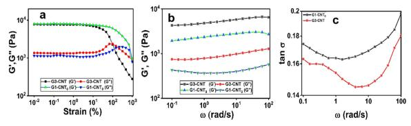
Fig. 3 Rheological investigation of G1-CNT<sub>0</sub> and G3-CNT hydrogels. (a) Strain sweep test, (b) frequency sweep test, and (c) damping factor elucidation.
