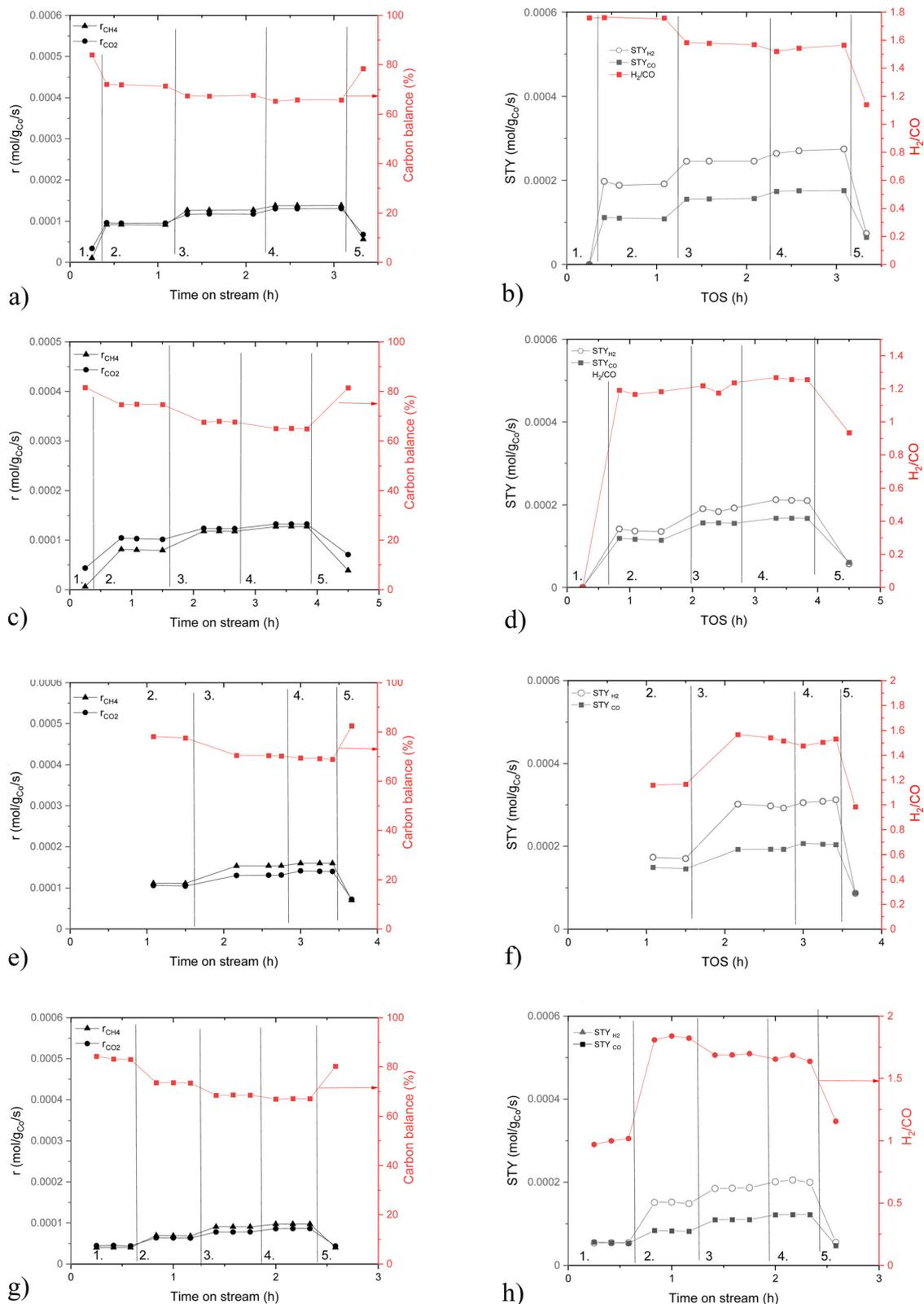
Fig. 7 Reaction rates for methane and CO<sub>2</sub> and carbon balance for (a) CoAl, (c) CoCeAl, (e) CoLaAl, and (g) CoCeLaAl and (b), (d), (f) and (h) the corresponding space time yields and H<sub>2</sub>/CO ratios for different catalysts. Notation: 1. 600 °C, 2. 700 °C, 3. 800 °C, 4. 900 °C and 5. 600 °C.
