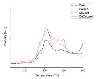
Fig. 4 Hydrogen TPR of all catalysts.
