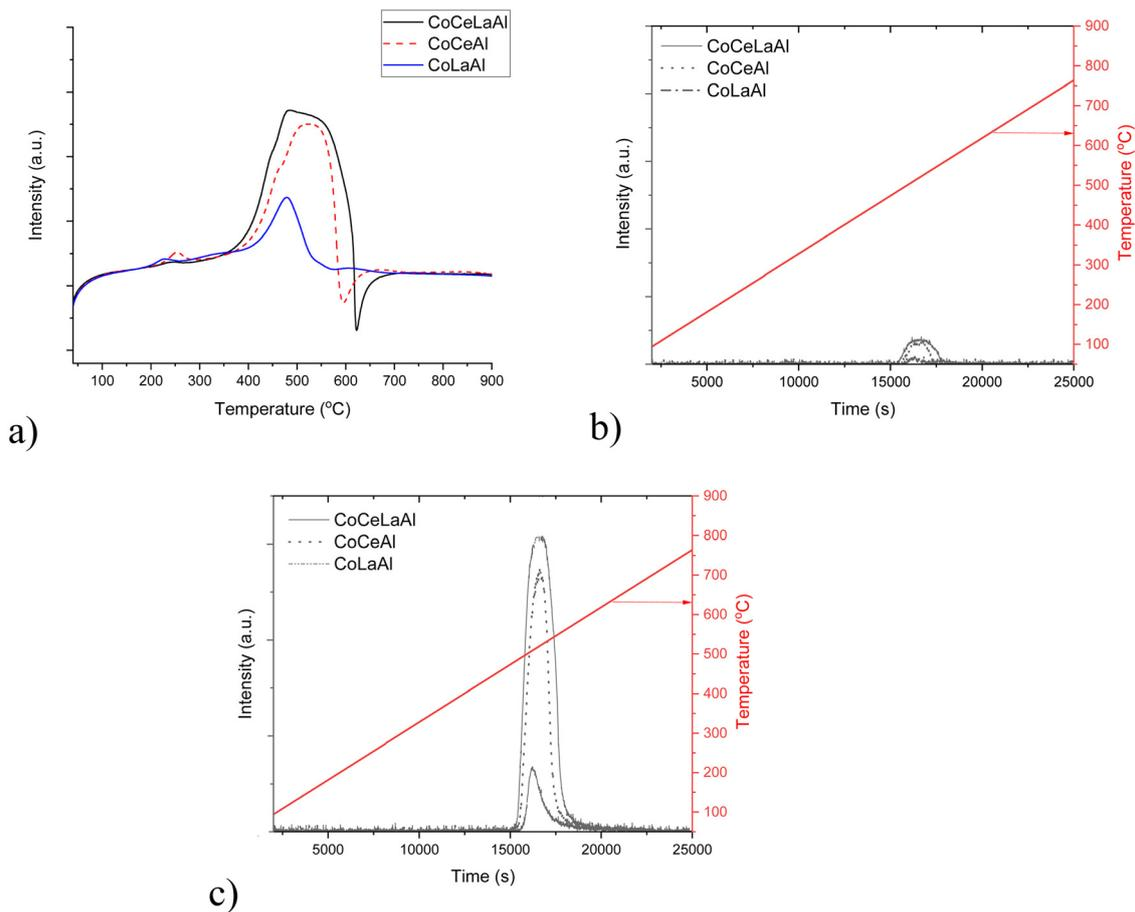
Fig. 6 (a) TCD signal, (b) formed CO and (c) CO<sub>2</sub> during temperature-programmed oxidation of spent catalysts.
