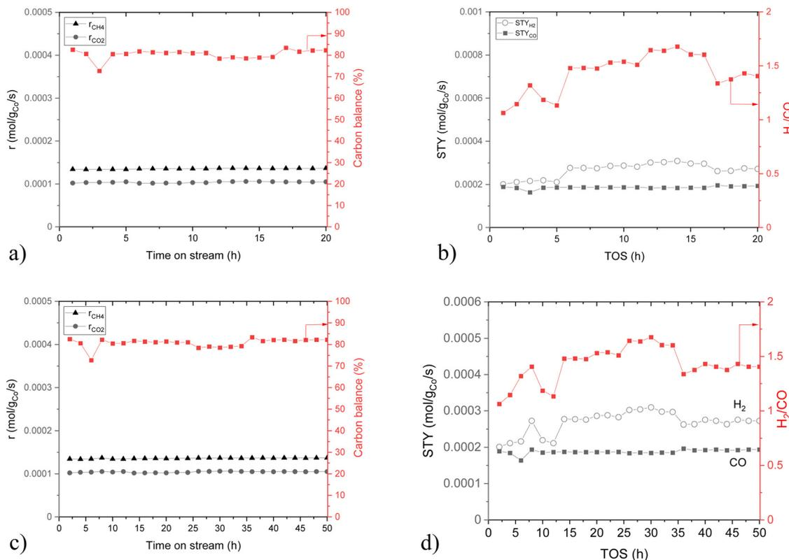
Fig. 9 Reaction rates for methane and CO<sub>2</sub> and carbon balance for CoLaAl for (a) 20 h and (c) 50 h TOS. (b) and (d) Corresponding space-time yields and H<sub>2</sub>/CO ratios for (b) 20 h and (d) 50 h TOS. Conditions: 800 °C, WHSV h<sup>-1</sup>.
