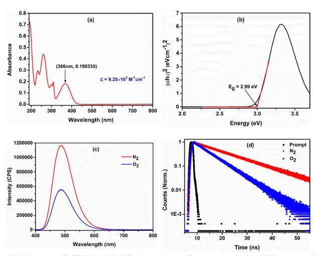
Fig. 2 (a) UV-visible spectrum of Ph-BT-Ph in acetonitrile. (b) Bandgap estimation using Tauc plot transformation. (c) and (d) Fluorescence and lifetime spectra of Ph-BT-Ph in acetonitrile.
