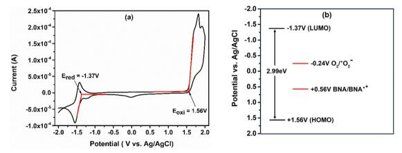
Fig. 3 (a) Cyclic voltammogram of Ph-BT-Ph in an acetonitrile solvent. (b) Schematic representation of the HOMO-LUMO position of Ph-BT-Ph relative to the reduction potential  $O_2/^{\bullet}O_2^{-}$  system and oxidation potential of benzylamine.
