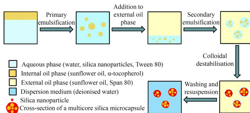
**Fig. 1** The preparation steps for the production of multicore silica microcapsules containing different concentrations of the internal oil phase, *i.e.* a mixture of  $\alpha$ -tocopherol and sunflower oil, through the salt-induced destabilisation of silica nanoparticles and their subsequent agglomeration in an O/W/O double emulsion template at room temperature.
