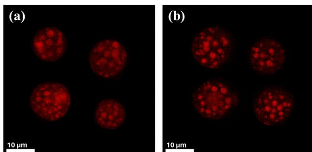
Fig. 6 Confocal microscopy images of multicore silica microcapsules containing 10 wt% of the internal oil phase, *i.e.* a mixture of  $\alpha$ -tocopherol and sunflower oil, which were prepared with 1 wt% of Span 80 in the external oil phase on the day of preparation (a) and after eight months (b).
