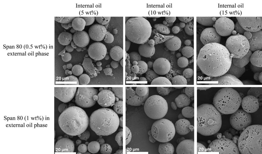
Fig. 4 SEM images of multicore silica microcapsules containing different concentrations of internal oil phase, *i.e.* a mixture of  $\alpha$ -tocopherol and sunflower oil, and prepared with different concentrations of Span 80 in the external oil phase.
