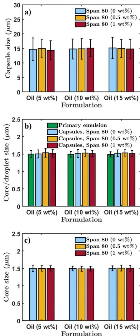
**Fig. 3** (a) Average size of multicore silica microcapsules containing different concentrations of the internal oil phase, *i.e.* a mixture of  $\alpha$ -tocopherol and sunflower oil, and prepared with different concentrations of Span 80 in the external oil phase. (b) Core size on the day of preparation and (c) core size six weeks post preparation. The error bars correspond to the standard deviation of 200 measured microcapsule diameters and 100 measured core diameters.
