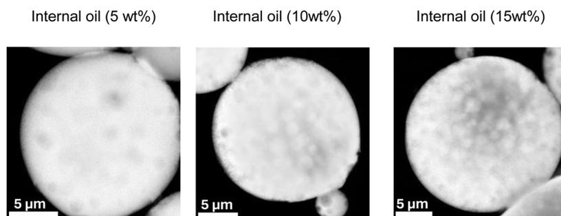
Fig. 5 Representative STEM images of multicore silica microcapsules containing different concentrations of internal oil, *i.e.* a mixture of  $\alpha$ -tocopherol and sunflower oil, which were prepared with 1 wt% of Span 80 in the external oil phase.
