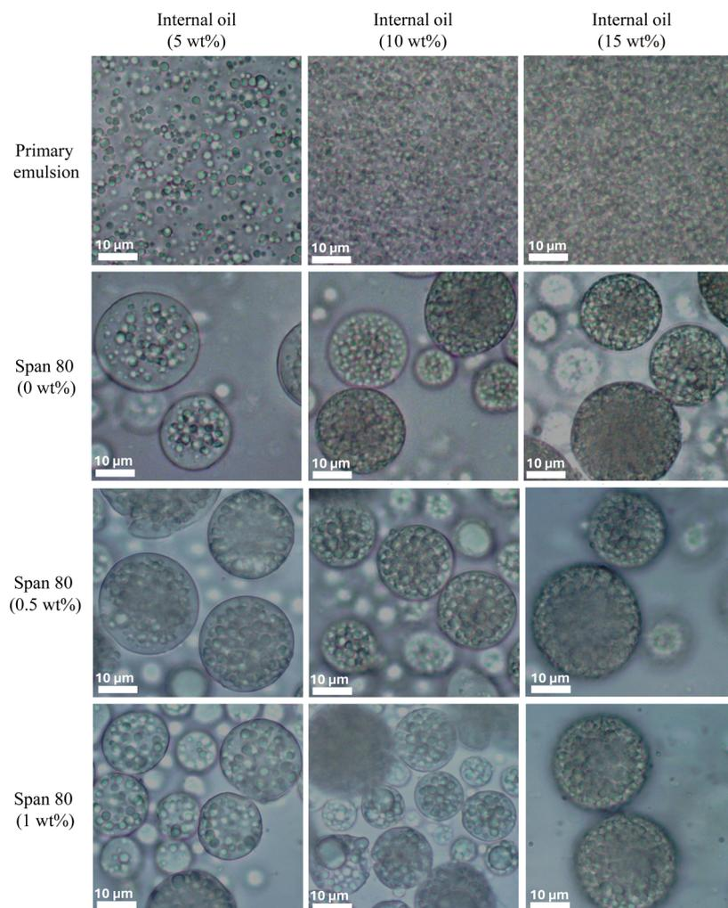
Fig. 2 Bright-field optical microscopy images of primary emulsions and the corresponding multicore silica microcapsules containing different concentrations of the internal oil phase, *i.e.* a mixture of  $\alpha$ -tocopherol and sunflower oil, and prepared with different concentrations of Span 80 in the external oil phase. The images were obtained on the day of preparation.
