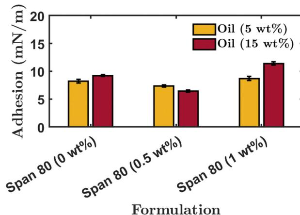
Fig. 8 Adhesion force of multicore silica microcapsules containing different concentrations of the internal oil phase, *i.e.* a mixture of  $\alpha$ -tocopherol and sunflower oil, and prepared with different concentrations of Span 80 in the external oil phase. Each error bar corresponds to the standard error of each sample.
