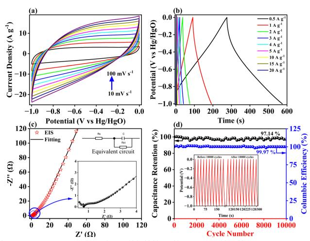
Electrochemical characterization of the KZAC sample: (a) CV, (b) GCD and (c) Nyquist plot of KZAC and (d) stability and capacitance retention.
