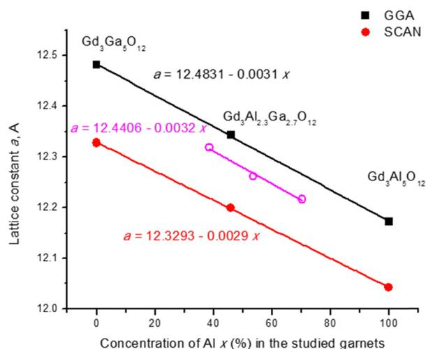
Fig. 11 Calculated (this work) lattice constants in  $\text{\AA}$  as a function of Al concentration (in %) in the studied garnets. Empty symbols show the experimental data from ref. 5. Equations of linear fits are shown.
