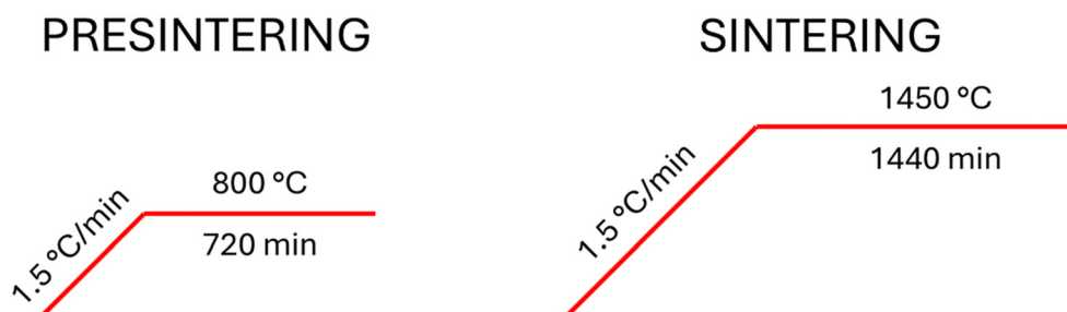
Fig. 1 Presintering and sintering temperature profiles of the rod precursor.
