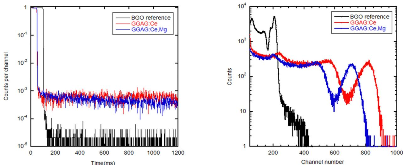
Fig. 6 RT spectrally unresolved afterglow curve of GGAG:Ce, GGAG:Ce,Mg and BGO standard, excitation by 40 kV X-ray (left) and pulse-height spectra for GGAG:Ce, GGAG:Ce,Mg and BGO under  $\gamma$ -ray excitation from  $^{137}\text{Cs}$  radioisotope (662 keV).
