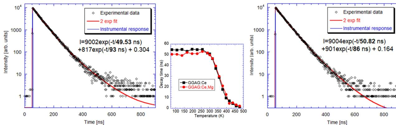
Fig. 8 RT photoluminescence decay curve connected to  $\text{Ce}^{3+} 4f \rightarrow 5d^1$  emission ( $\lambda_{\text{ex}} = 454 \text{ nm}$ ,  $\lambda_{\text{em}} = 530 \text{ nm}$ ) of GGAG:Ce (left) and GGAG:Ce,Mg (right). Solid line is a convolution of the instrumental response and function  $I(t)$  in the figure. In the inset, the temperature dependence of the faster component decay time is shown for both samples.
