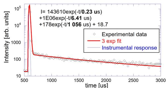
Fig. 9 PL decay of the  $\text{Gd}^{3+}$  312 nm emission line under excitation at 275 nm.
