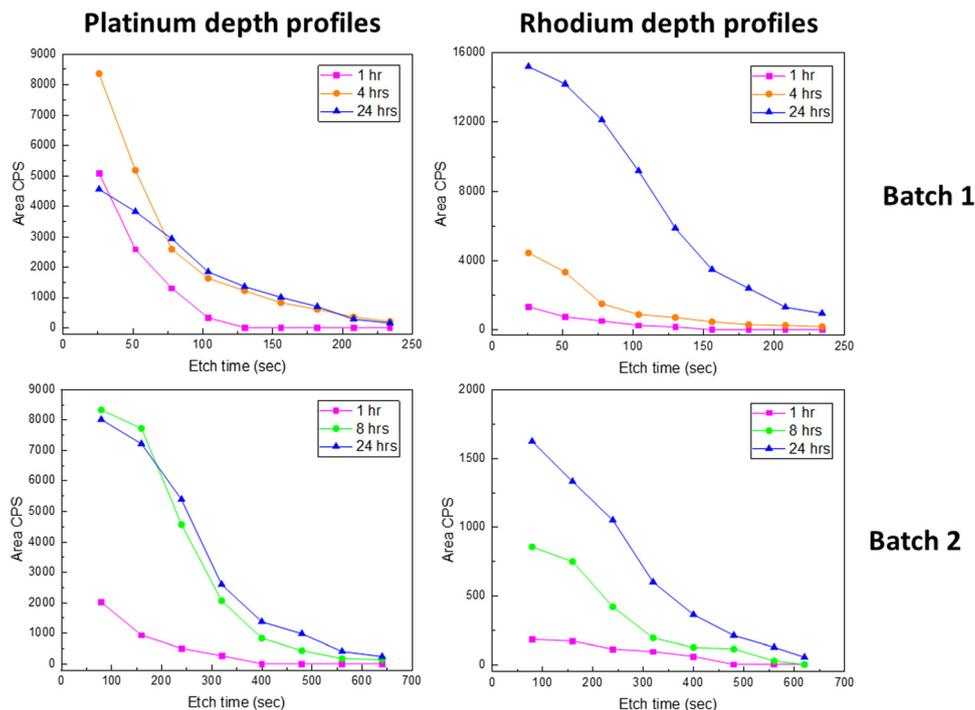
Fig. 6 Platinum depth profiles and rhodium depth profiles in LNO films (without post-annealing) after 1, 4 (batch 1)/8 (batch 2) and 24 h  $\text{PtO}_2(\text{g})$  and  $\text{RhO}_2(\text{g})$  exposure, shown with the area CPS of Pt  $4d_{3/2}$  and Rh  $3d_{5/2}$  for batch 1 and batch 2.
