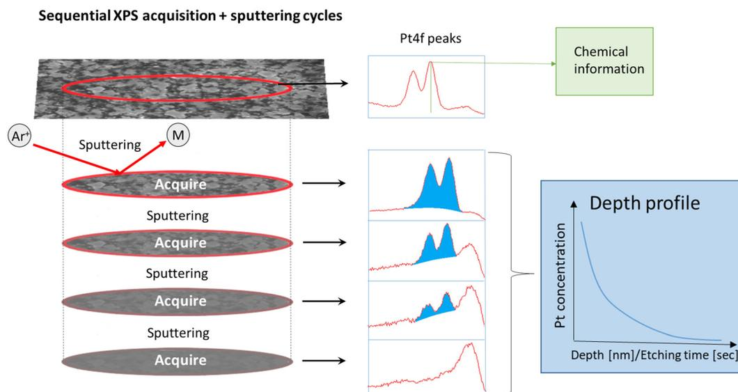
Fig. 1 Illustration of sequential Ar<sup>+</sup> sputtering and XPS collection of ALD thin films.
