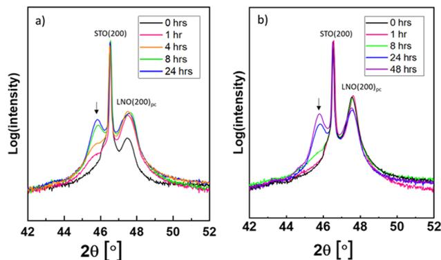
Fig. 2 Powder X-ray diffractograms of LNO films on STO substrates after  $\text{PtO}_2(\text{g})$  exposure for various durations, see (a) without post-annealing and (b) with post-annealing. The emerging peaks ascribed to  $\text{La}_2\text{NiPtO}_6$  are marked by arrows. The Bragg reflections (200) for STO and pseudocubic (200) for LNO are ascribed to the other peaks in the diffractograms.
