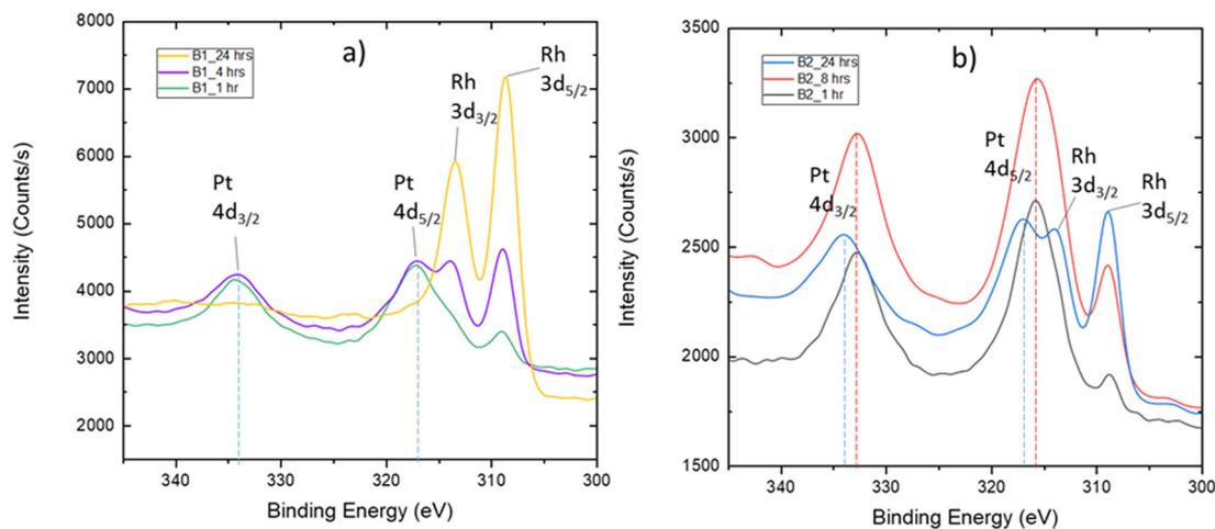
**Fig. 5** XPS narrow scans of LNO surfaces after simultaneous exposure to  $\text{PtO}_2(\text{g})$  and  $\text{RhO}_2(\text{g})$  for (a) 1, 4 and 24 h in the case of batch 1 (B1) and for (b) 1, 8 and 24 h in the case of batch 2 (B2).
