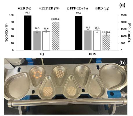
Fig. 9 (a) Aerodynamic dispersion parameters of TQ and DOX from TQ-DOX/Cys-Py/PA NCs; ED: emitted dose; FPF-ED: fine particle fraction of emitted dose; FPF-TD: fine particle fraction of theoretical dose; and RD: respirable dose. Results are presented as mean  $\pm$  SD, n = 3 and (b) the deposition of the TQ and DOX aggregates of TQ-DOX/Cys-Py/PA NCs onto the NGI trays as orange powder from tray 1 to tray 7.
