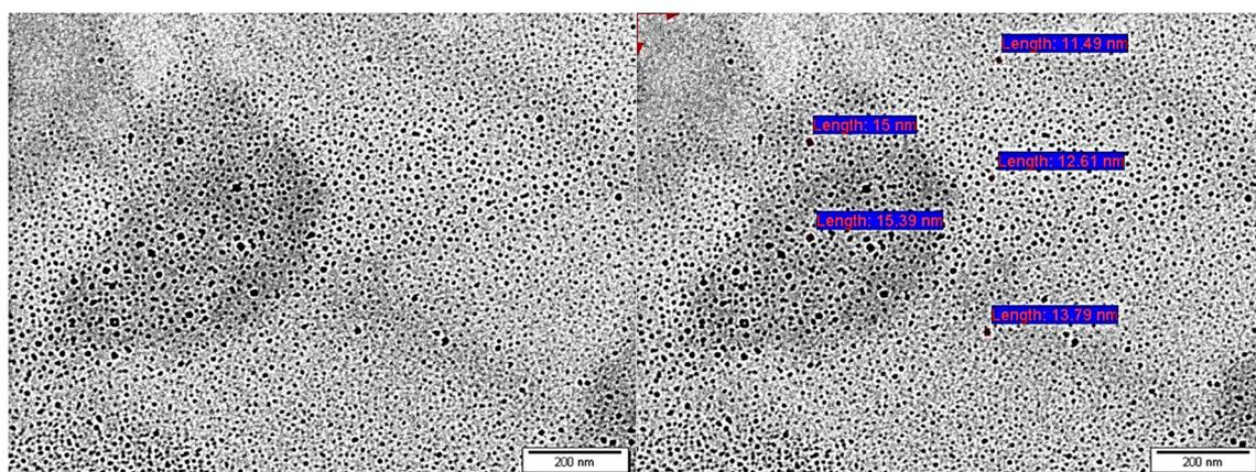
Fig. 7 TEM micrographs of TQ-DOX/Cys-Py/PA NCs highlighting the particle shape and size. Scale bar = 200 nm.
