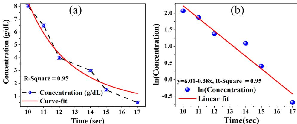
Fig. 7 Reaction kinetic study on prepared  $\mu\text{PADs}$ : (a) formation of a blue-molybdenum complex as a function of time, and (b) a linear relationship between  $\ln(\text{concentration})$  and time, indicating first-order reaction kinetics with a downward slope.
