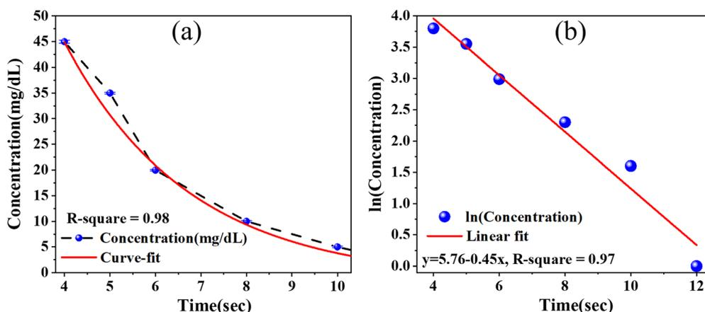
Fig. 6 Reaction kinetic study on prepared  $\mu\text{PADs}$ : (a) Formation of a pink-colored complex as a function of time, and (b) A linear relationship between  $\ln(\text{concentration})$  and time, indicating first-order reaction kinetics with a downward slope.
