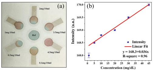
Fig. 4 (a) Concentration based colorimetric detection of zinc in artificial soil solutions on μPADs. (b) Quantitative Analysis studied by calibration curve generated for the range of 1 mg dL<sup>-1</sup> to 45 mg dL<sup>-1</sup> zinc by measuring the intensity of color formed in detection reservoirs.
