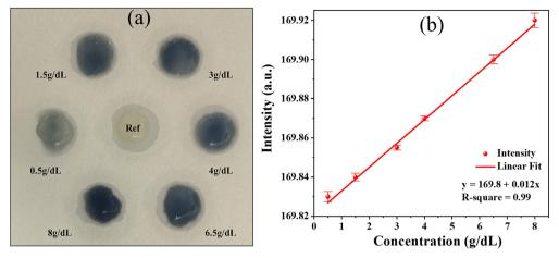
Fig. 5 (a) Concentration based colorimetric detection of orthophosphate in artificial soil solutions on paper μPADs. (b) Quantitative analysis studied by calibration curve generated for the range of 0.5-8 g dL $^{-1}$  orthophosphate by measuring the intensity of color formed in detection reservoirs.
