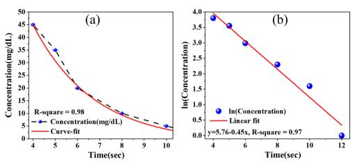
Fig. 6 Reaction kinetic study on prepared μPADs: (a) Formation of a pink-colored complex as a function of time, and (b) A linear relationship between ln (concentration) and time, indicating first-order reaction kinetics with a downward slope.
