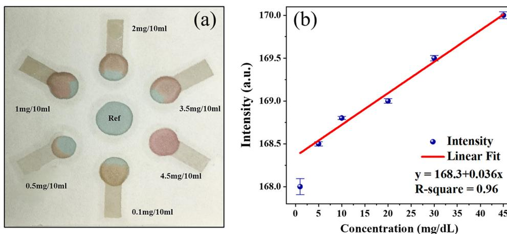
Fig. 4 (a) Concentration based colorimetric detection of zinc in artificial soil solutions on  $\mu\text{PADs}$ . (b) Quantitative Analysis studied by calibration curve generated for the range of  $1 \text{ mg dL}^{-1}$  to  $45 \text{ mg dL}^{-1}$  zinc by measuring the intensity of color formed in detection reservoirs.
