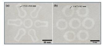
Fig. 1 Analysis of the width measurement in the prepared μPADs for (a) zinc and (b) orthophosphate colorimetric sensing.
