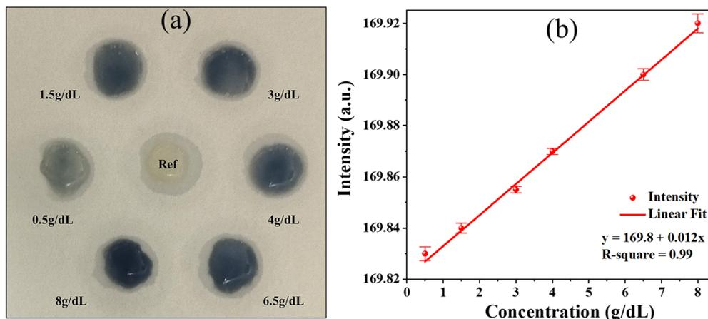
Fig. 5 (a) Concentration based colorimetric detection of orthophosphate in artificial soil solutions on paper  $\mu$ PADs. (b) Quantitative analysis studied by calibration curve generated for the range of 0.5–8  $\text{g dL}^{-1}$  orthophosphate by measuring the intensity of color formed in detection reservoirs.
