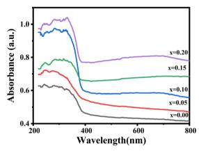
Fig. 8 UV-Vis absorption spectra of  $BaTi_{1-x}Zr_xO_3$  ceramics versus the wavelength of incident photons.
