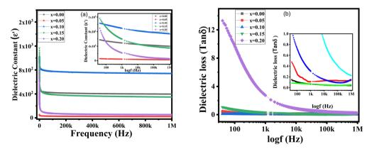
Fig. 6 Frequency-dependent dielectric properties of  $BaZr_xTi_{1-x}O_3$  ceramics: (a) dielectric constant; (b) dielectric loss  $(\tan\delta)$ . The inset shows the enlarged view.
