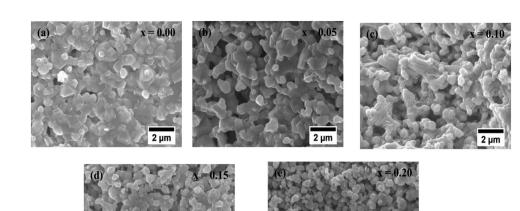
Fig. 4 FE-SEM micrographs of the synthesized BZT ceramics with different compositions: (a) x = 0.00, (b) x = 0.05, (c) x = 0.10, (d) x = 0.15, and (e) x = 0.20.
