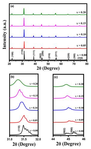
Fig. 1 (a) XRD patterns of  $BaZr_xTi_{1-x}O_3$  (x = 0.00, 0.05, 0.10, 0.15, and0.20), (b) magnified pattern of the (110) peaks around  $2\theta = 31^{\circ}$ , and (c) (002) (200) peaks illustrating a shift at around  $2\theta = 45^{\circ}$  for various x contents
