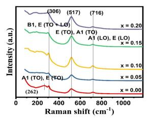
Fig. 3 Raman spectra of  $BaZr_xTi_{1-x}O_3$  ceramics (x = 0.00, 0.05, 0.10, 0.15, and 0.20).
