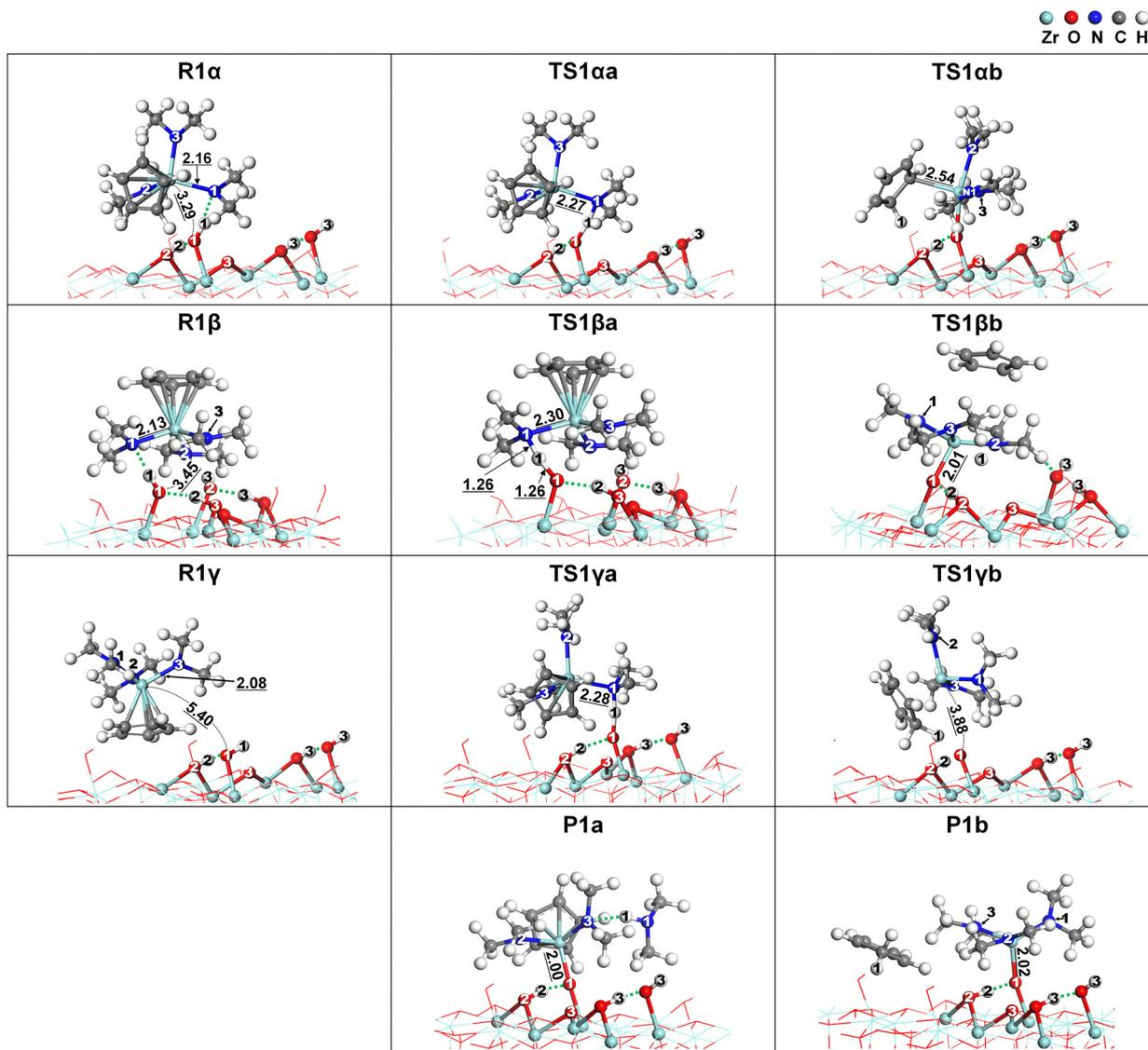
Fig. 7 The atomistic structural changes for the paths from three reactant states, **R1 $\alpha$** , **R1 $\beta$** , and **R1 $\gamma$** , to two product states, **P1a** and **P1b**. The dotted lines indicate hydrogen bonds. Bond lengths are given in Å.
