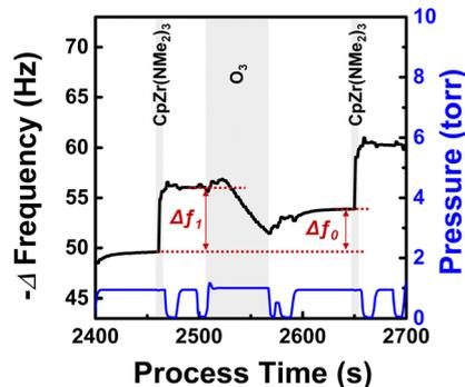
Fig. 3 Change in resonance frequency throughout the  $\text{ZrO}_2$  ALD process at 230 °C.  $\text{CpZr}(\text{NMe}_2)_3$  and  $\text{O}_3$  were alternately supplied with pulse times of 7 s and 60 s, respectively.
