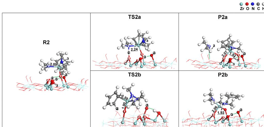
Fig. 8 The atomistic structural changes for the paths from **R2** to two product states, **P2a** and **P2b**. The dotted lines indicate hydrogen bonds. Bond lengths are given in Å.
