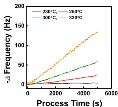
Fig. 2 Resonance frequency change resulting from repeated  $\text{CpZr}(\text{NMe}_2)_3$  pulses and Ar purges in the absence of the  $\text{O}_3$  supply. Process temperature was varied to identify the onset of the thermal decomposition of the precursor.
