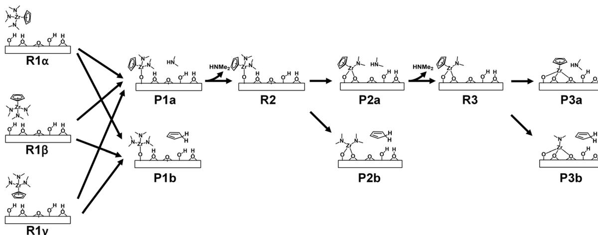
**Fig. 4** Schematic of the multiple paths of surface reactions of CpZr(NMe<sub>2</sub>)<sub>3</sub> on the ZrO<sub>2</sub> substrate.
