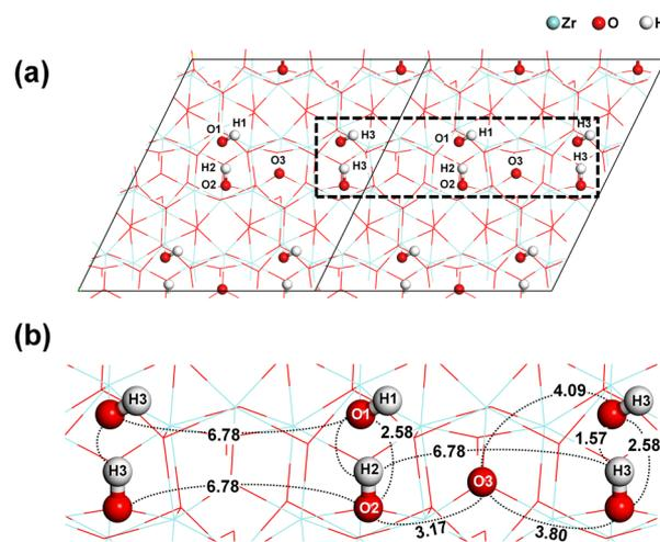
Fig. 1 Schematic illustration of (a) the monoclinic  $\text{ZrO}_2$  ( $-111$ ) slab model and (b) the reaction sites considered for the chemisorption of Zr precursor. Interatomic distances are given in Å.
