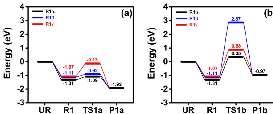
Fig. 5 Energy diagrams for the first reaction of CpZr(NMe<sub>2</sub>)<sub>3</sub> from three reactant states, R1 $\alpha$ , R1 $\beta$ , and R1 $\gamma$ , to two product states, (a) P1a and (b) P1b.
