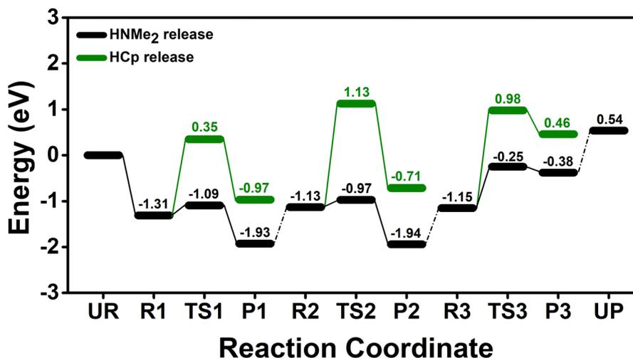
Fig. 6 Energy diagrams for the surface reactions of CpZr(NMe<sub>2</sub>)<sub>3</sub> on ZrO<sub>2</sub>. The P<sub>na</sub> states are the product states resulting from the *n*th surface reaction with the release of HNMe<sub>2</sub>, while the P<sub>nb</sub> states are the product states arising from the release of HCp.
