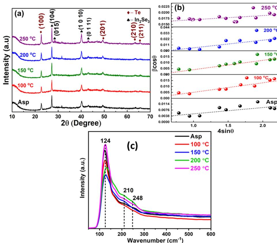
Fig. 6 (a) XRD pattern and (b) Williamson–Hall plot (c) Raman spectra of as-prepared and annealed Te/In<sub>2</sub>Se<sub>3</sub> thin films.
