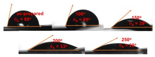
Fig. 11 Contact angle pictures of Te/In<sub>2</sub>Se<sub>3</sub> thin films.
