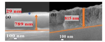
Fig. 1 Cross-sectional FESEM image of Te/In<sub>2</sub>Se<sub>3</sub> (a) as-prepared (b) 250 °C annealed film.
