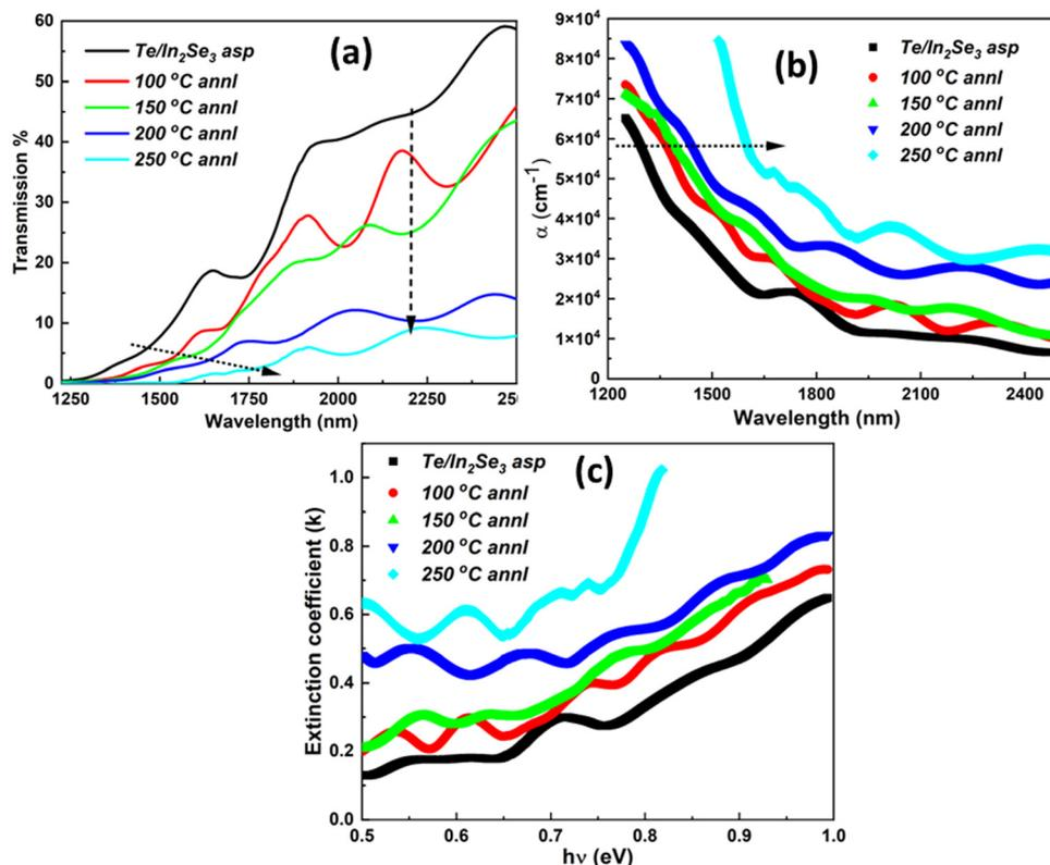
Fig. 8 (a) Transmission (b) absorption coefficient (c) extinction coefficient of the Te/In<sub>2</sub>Se<sub>3</sub> film.
