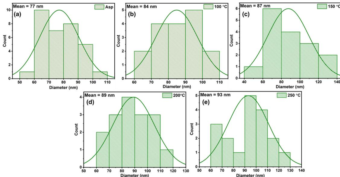
Fig. 4 Particle size distribution of Te/In<sub>2</sub>Se<sub>3</sub> films at different conditions.
