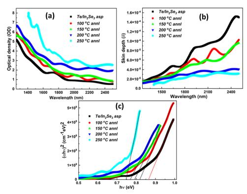
(a) Optical density (b) skin depth (c) bandgap of the Te/In<sub>2</sub>Se<sub>3</sub> film.
