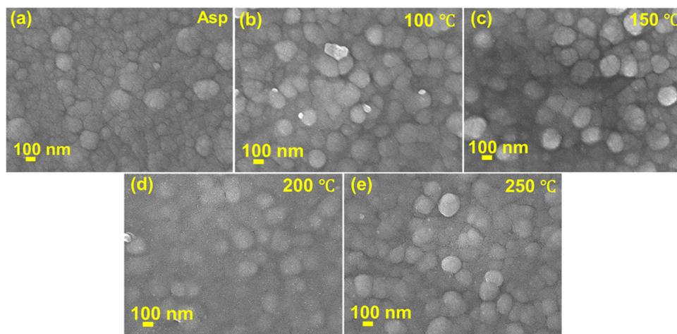
Fig. 3 FESEM images of Te/In<sub>2</sub>Se<sub>3</sub> films at different conditions at 100 nm.
