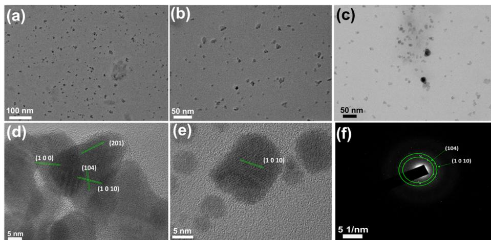
Fig. 5 (a)–(c) TEM images, (d) and (e) HRTEM images, and (f) SAED pattern of the 250 °C annealed Te/In<sub>2</sub>Se<sub>3</sub> thin films.
