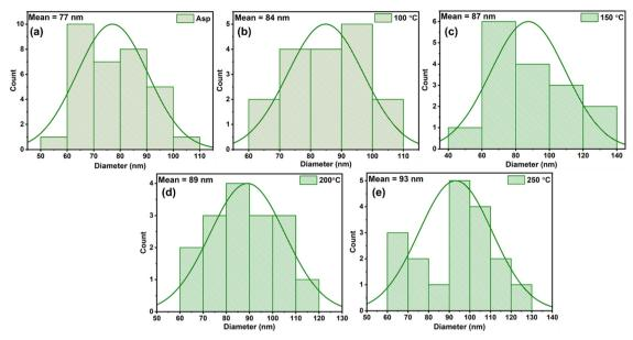
Fig. 4 Particle size distribution of Te/In<sub>2</sub>Se<sub>3</sub> films at different conditions
