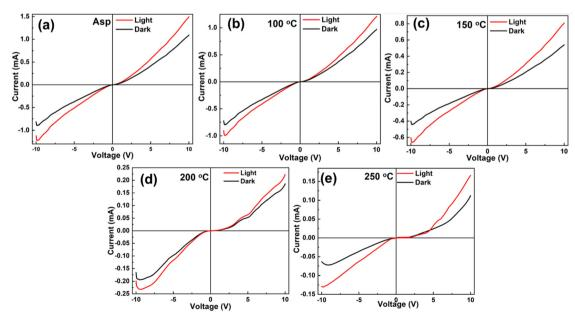
Fig. 13 Individual I-V characteristics plot (a) as-prepared, (b) 100 °C, (c) 150 °C, (d) 200 °C, and (e) 250 °C under dark and light conditions of Te/In<sub>2</sub>Se<sub>3</sub> thin films.
