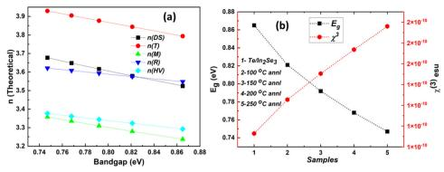
Fig. 10 (a) Theoretical refractive index variation with bandgap (b) variation of  $\gamma^{(3)}$  and bandgap for different samples.
