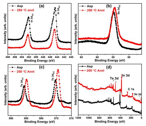
Fig. 7 XPS spectra of (a) In 3d, (b) Se 3d, and (c) Te 3d (d) survey spectra of as-prepared and 250 °C annealed Te/In<sub>2</sub>Se<sub>3</sub> thin film.
