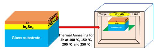
Scheme 1 Schematics of Te/In<sub>2</sub>Se<sub>3</sub> film and annealing procedure
