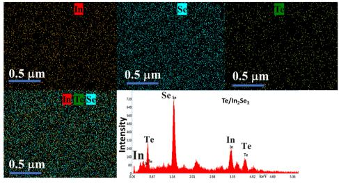
Fig. 2 EDX mapping and spectra of as-prepared Te/In<sub>2</sub>Se<sub>3</sub> film.
