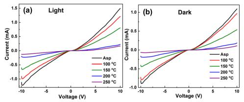
Fig. 12 I-V characteristics plot (a) light and (b) dark for the Te/In<sub>2</sub>Se<sub>3</sub> thin films.
