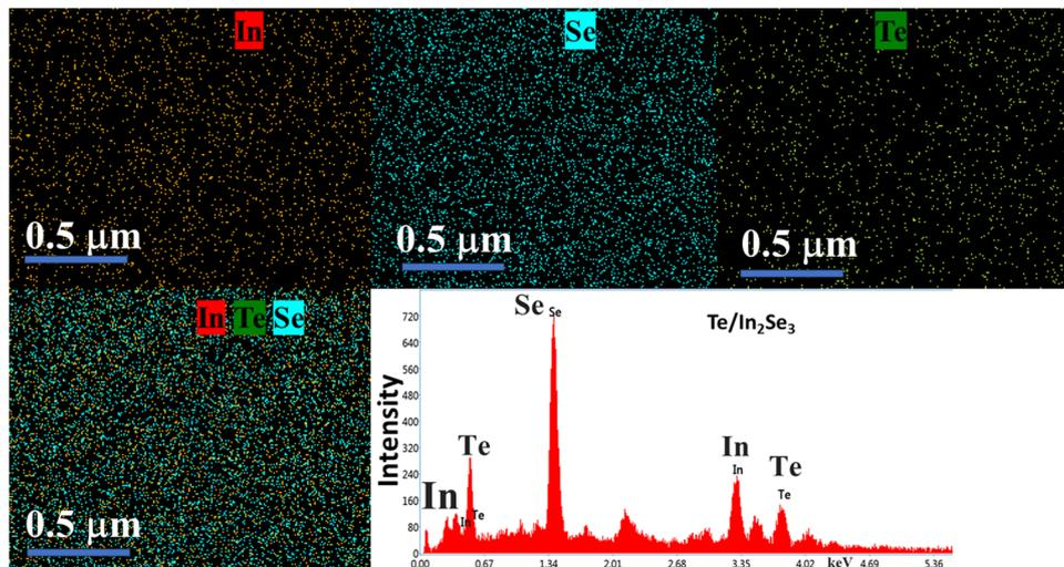
Fig. 2 EDX mapping and spectra of as-prepared Te/In<sub>2</sub>Se<sub>3</sub> film.
