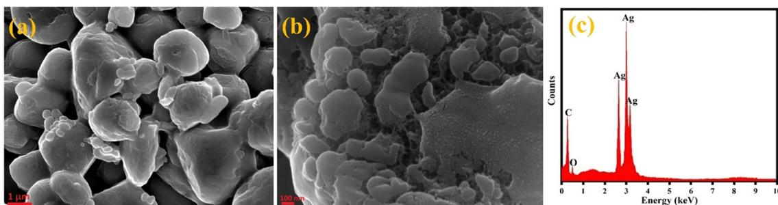
Fig. 4 SEM micrographs at (a) 1  $\mu\text{m}$  (b) 100 nm and (c) EDX spectrum of  $TGRAgNPs$ .
