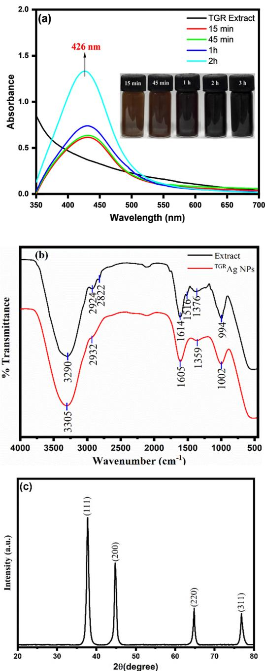
Fig. 3 (a) UV-visible spectra of TGR extract and TGR extract synthesised AgNPs (Inset: optical images of  $\text{TGR Ag NPs}$  at different time intervals), (b) FTIR spectra and (c) XRD diffractogram of  $\text{TGR Ag NPs}$ .
