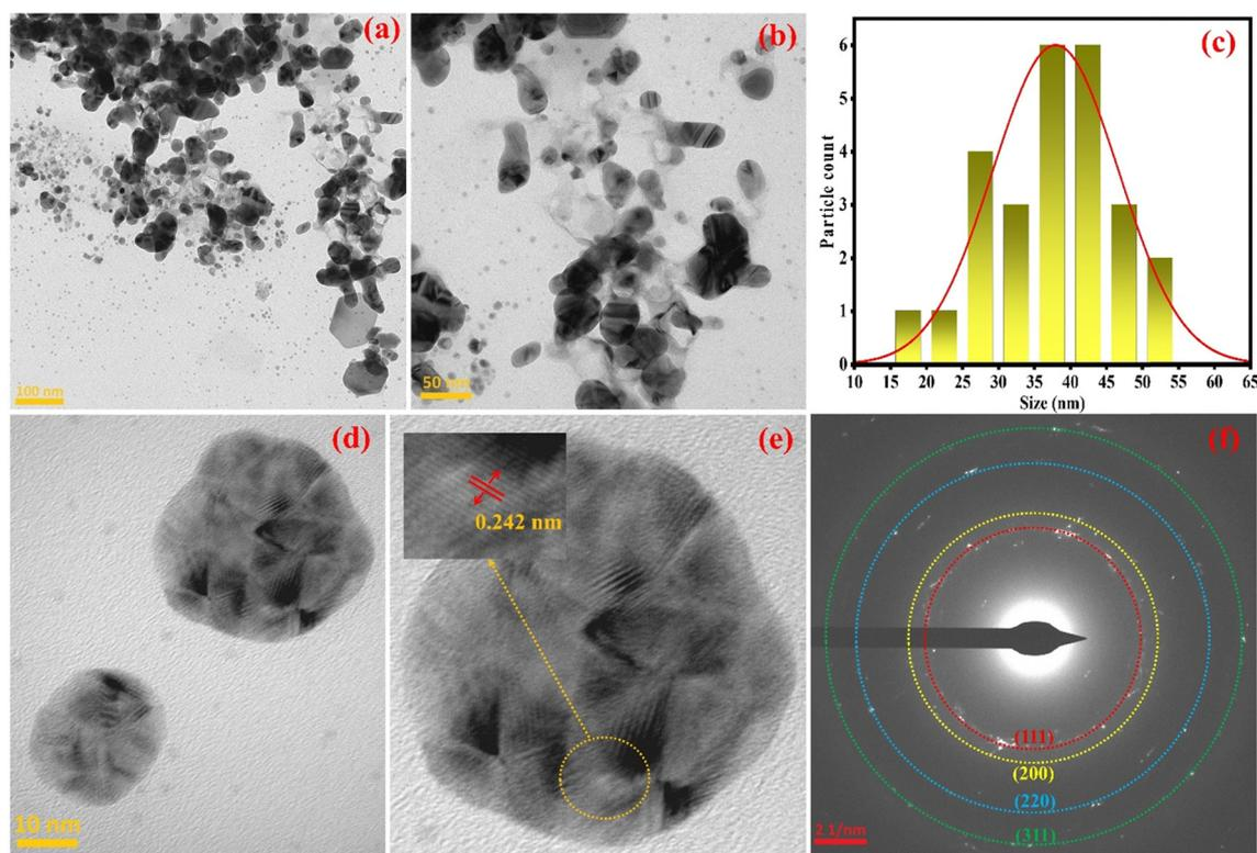
Fig. 5 TEM micrographs at (a) 100 nm (b) 50 nm nanoscale magnifications, (c) size distribution histogram, (d) HR-TEM (e) HR-TEM with zoom-in showing lattice fringes and (f) SAED patterns of  $TGR-AgNPs$ .
