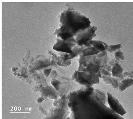
Fig. 3 TEM image of the  $\text{Bi}_{1.75}\text{La}_{0.25}\text{FeMnO}_6$  ceramic.
