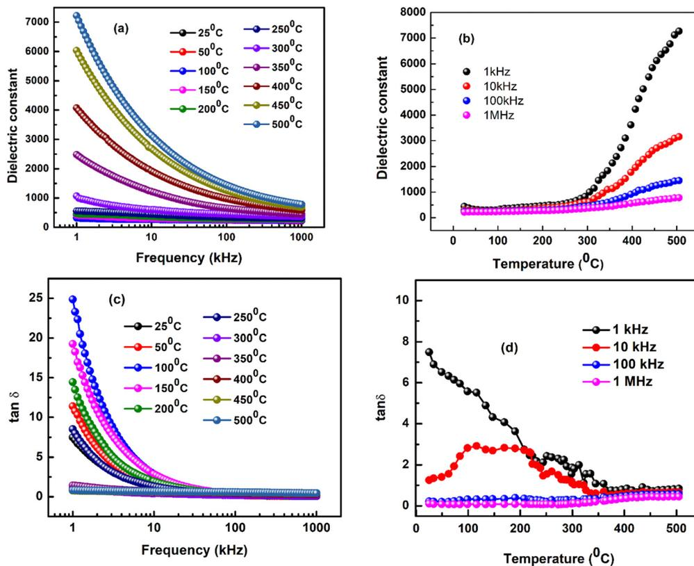
Fig. 6 (a) Dielectric constant versus frequency, (b) dielectric constant versus temperature of the  $\text{Bi}_{1.75}\text{La}_{0.25}\text{FeMnO}_6$  ceramic. (c)  $\tan \delta$  versus frequency and (d)  $\tan \delta$  versus temperature of the  $\text{Bi}_{1.75}\text{La}_{0.25}\text{FeMnO}_6$  ceramic.
