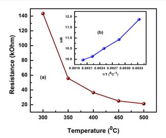
Fig. 10 (a) Resistance versus temperature and (b)  $1/T\ versus\ \ln R$  of the BLFMO ceramic.
