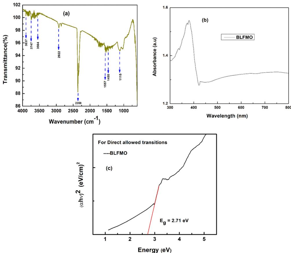
Fig. 5 (a) FTIR, (b) absorbance spectrum, and (c) energy versus  $(\alpha h\nu)^2$  for direct allowed transitions to calculate the bandgap energy of the  $\text{Bi}_{1.75}\text{La}_{0.25}\text{FeMnO}_6$  ceramic.
