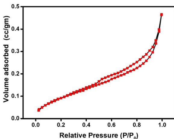
Fig. 4 Nitrogen sorption isotherms of the compound  $\text{Bi}_{1.75}\text{La}_{0.25}\text{FeMnO}_6$ .
