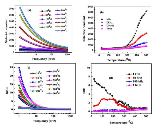
Fig. 6 (a) Dielectric constant versus frequency, (b) dielectric constant versus temperature of the Bi<sub>1.75</sub>La<sub>0.25</sub>FeMnO<sub>6</sub> ceramic. (c)  $\tan \delta$  versus frequency and (d)  $\tan \delta$  versus temperature of the Bi<sub>1.75</sub>La<sub>0.25</sub>FeMnO<sub>6</sub> ceramic.
