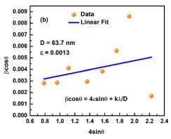
Fig. 1 (a) XRD pattern analysis and (b) Williamson-Hall plot of the Bi<sub>1.75</sub>La<sub>0.25</sub>FeMnO<sub>6</sub> ceramic.
