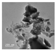
Fig. 3 TEM image of the Bi<sub>1.75</sub>La<sub>0.25</sub>FeMnO<sub>6</sub> ceramic
