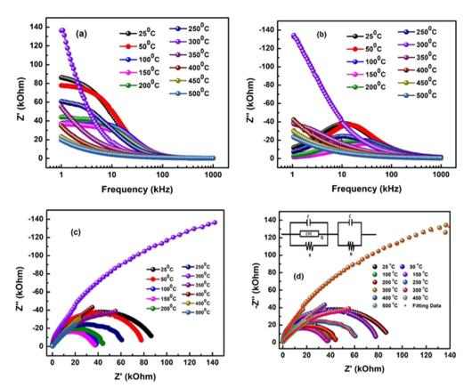
Fig. 7 (a) Z' versus frequency, (b) Z" versus frequency, (c) Nyquist plot, and (d) fitted Nyquist plots of the Bi<sub>1.75</sub>La<sub>0.25</sub>FeMnO<sub>6</sub> ceramic.
