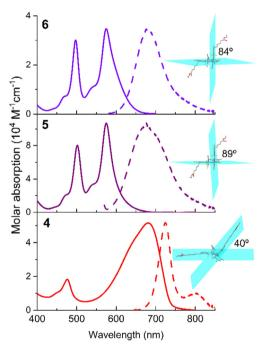
Fig. 5 Absorption and normalized fluorescence (dashed) spectra of 3-3' BODIPY dimer 4 and its corresponding constrained brominated (5) and methylated (6) derivatives in chloroform (dye concentration 2  $\mu$ M). The corresponding ground optimized geometries are also appended, highlighting the torsional angles between the chromophoric planes. The corresponding spectra in more solvents are recorded as shown in Fig. S20 and S21 of the ESI.†
