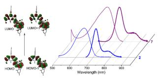
Fig. 4 Normalized absorption (thin line) and fluorescence (thick line) spectra of representative 3-3' BODIPY dimers 2 and 7 (dye concentration  $2 \mu M$ ) in acetonitrile to highlight the photoactive spectral region covered with these dimers. The corresponding HOMO and LUMO contour maps of representative dimer 2 are also included. The rest of spectra in more solvents and for the other dimers are collected in Fig. S19-S21 in the ESI.†
