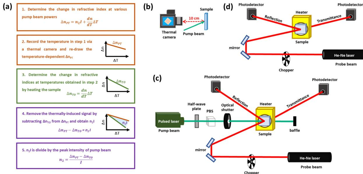
Fig. 3 (a) Flowchart of the process for estimating  $n_2$  values. (b) Experiment setup of the thermal camera system. (c) Pump-probe spectroscopy for assessing the degree of the photothermal nonlinearity. (d) Pump-probe setup for thermally induced nonlinearity.
