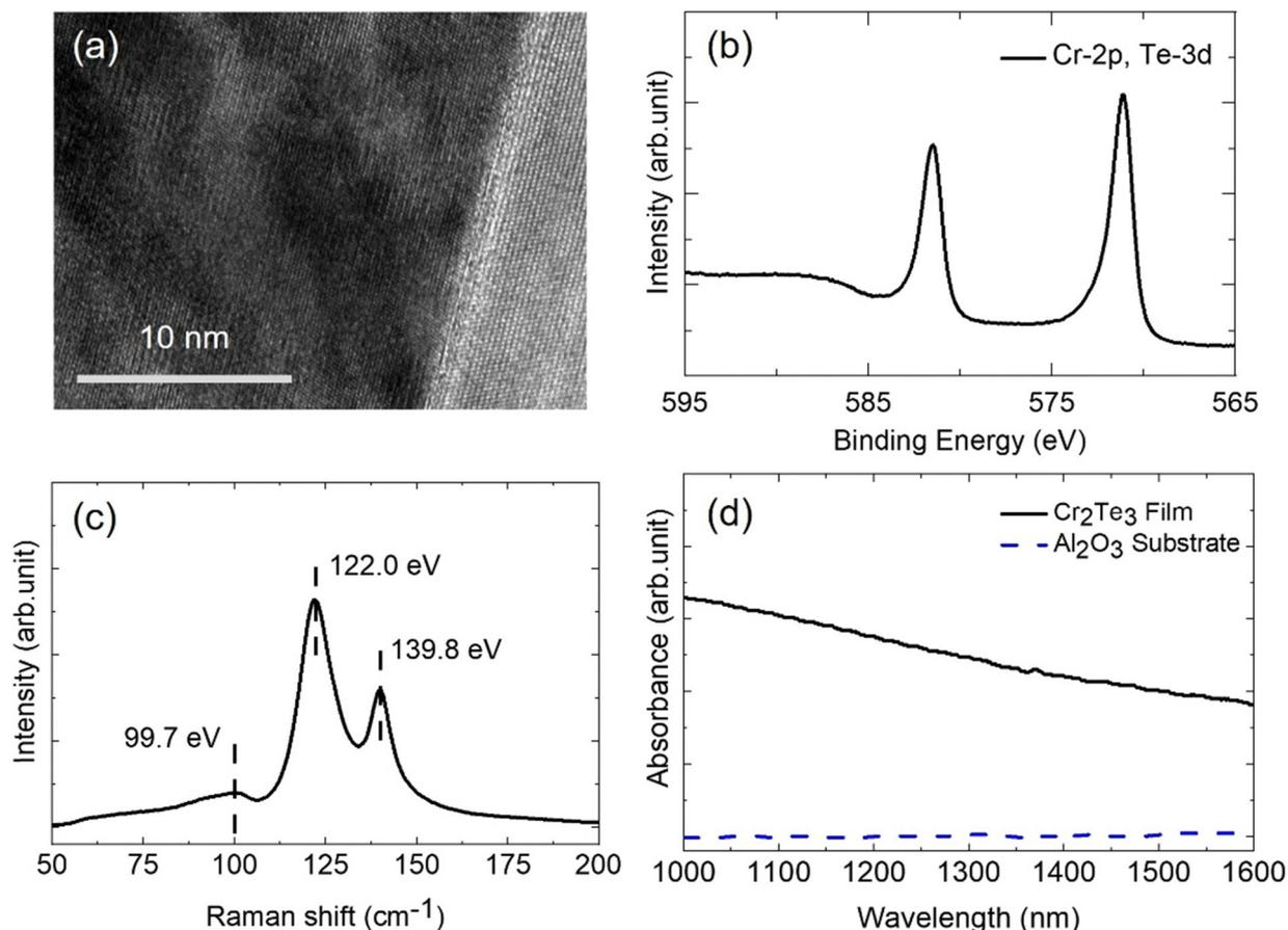
Fig. 1 (a) High-resolution TEM image, (b) XPS spectrum, (c) Raman spectrum, and (d) linear absorption spectrum of the Cr<sub>2</sub>Te<sub>3</sub> film.
