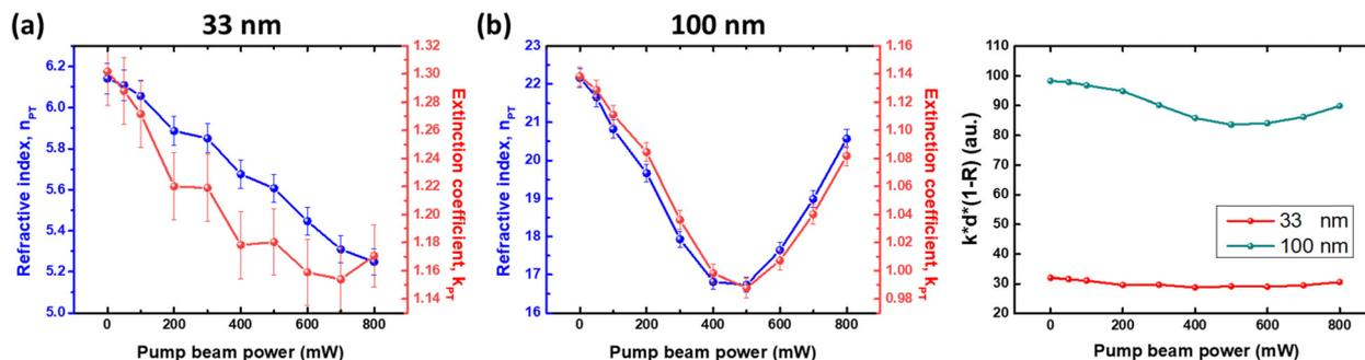
Fig. 6 (a) Power-dependent refractive index and extinction coefficient for 33-nm-thick and (b) 100-nm-thick  $\text{Cr}_2\text{Te}_3$  thin films; (c) estimated merit of absorption for the  $\text{Cr}_2\text{Te}_3$  thin films.
