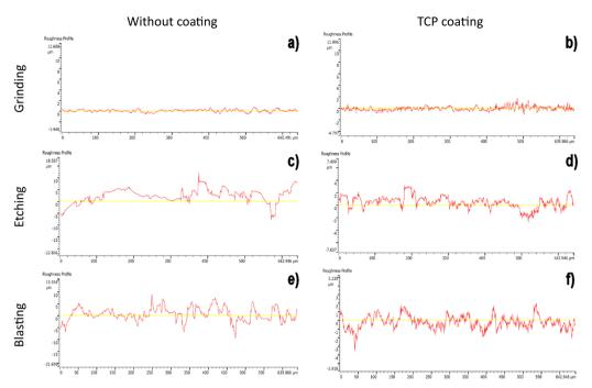
Fig. 4 Roughness profiles of mechanically and chemically treated substrates without coating and with TCP coating.
