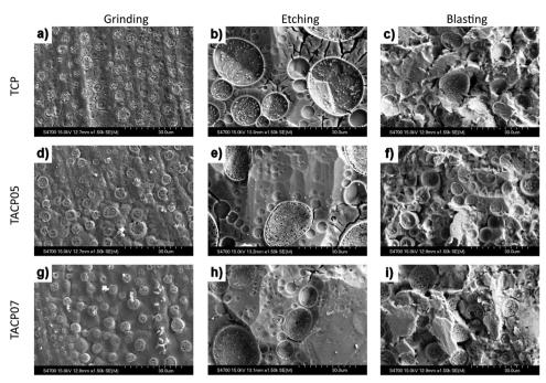
Fig. 2 SEM images of fired coatings surfaces
