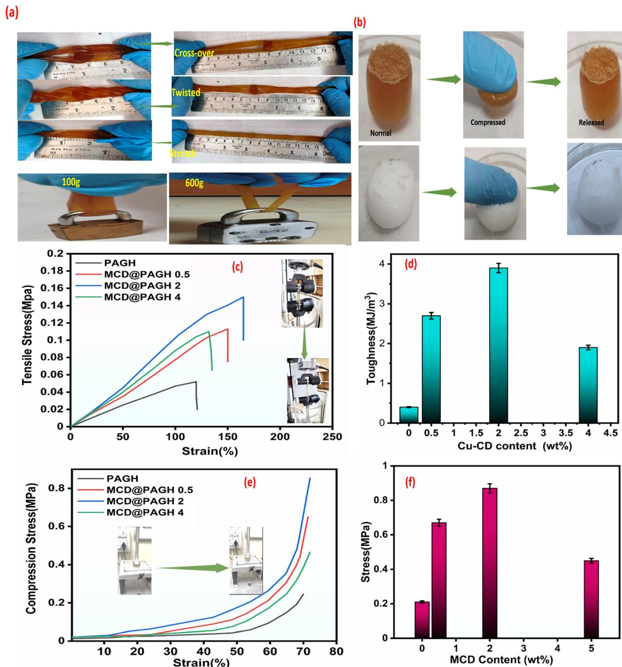
Fig. 2 (a) Photos of the stretching of the MCD@PAGH. (a) Crossover stretching, twisting and stretching between two MCD@PAGH, holding a weight of 100–600 g for the MCD@PAGH. (b) Compression image of MCD@PAGH and PAGH. (c) Tensile stress–strain plot. (d) Toughness of MCD@PAGH with different MCDs wt%. (e) Compressive stress–strain plot. (f) Compressive stress at 73% strain of MCD@PAGH with different MCD wt%.
