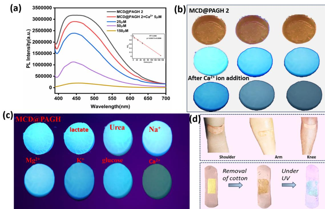
Fig. 6 (a) Hydrogel patch under day light. (b)  $\text{Ca}^{2+}$  detection in artificial sweat by hydrogel patch under UV (365 nm) light. (c) RGB app-based linear fitting of hydrogel patch. (d) Selectivity study of hydrogel patch compared to other metabolites and ions in sweat. (e) Hydrogel-based band-aid attached to shoulder, arm, knee.
