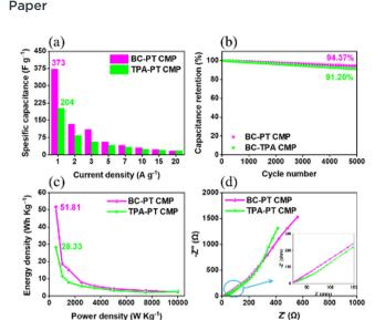
Fig. 6 (a) Specific capacitances of BC-PT and TPA-PT CMPs recorded at specific current densities (1.0 to 20 A  $g^{-1}$ ). (b) Cycling stability at 10 A  $g^{-1}$ current density over 5000 cycles. (c) Ragone plots. (d) Nyquist plots of cells with the as-synthesized polymers in a three-electrode system.
