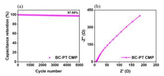
Fig. 9 (a) Cycling retention recorded at 10 A  $\rm g^{-1}$  current density over 5000 cycles; (b) Nyquist plot of the BC-PT polymer in a coin cell.
