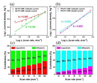
Fig. 7 (a) and (b) log(i) versus log(v) plots of (a) BC-PT, and (b) TPA-PT CMPs. (c) and (d) Relative contributions of the capacitive and diffusioncontrolled energy storage of (c) BC-PT, and (d) TPA-PT polymers, measured at various scan rates
