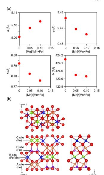
Fig. 4 (a) Change in lattice parameters of ε-Mn<sub>x</sub>Fe<sub>2-x</sub>O<sub>3-x/2</sub>. (b) Crystal structure of ε-Mn<sub>x</sub>Fe<sub>2-x</sub>O<sub>3-x/2</sub>. Orange, blue, green, purple, and red balls represent metal atoms at the A, B, C, and D sites, and O atoms, respectively.
