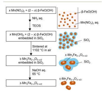
Fig. 1 Schematic of  $\varepsilon$ -Mn<sub>x</sub>Fe<sub>2-x</sub>O<sub>3-x/2</sub> nanoparticle synthesis.
