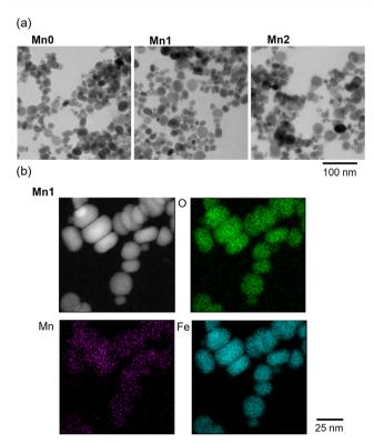
Fig. 2 (a) TEM images of Mn0, Mn1, and Mn2. (b) STEM-EDS images with elemental mapping of Mn1.
