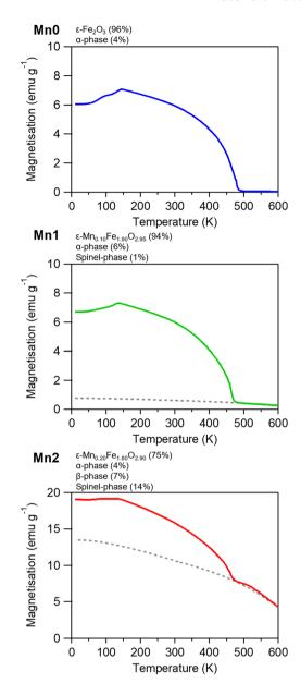
Fig. 5 FCM curves in an external field of 1 kOe for Mn0, Mn1, and Mn2. Dotted line is to guide the eye for the contribution of the spinel-phase.
