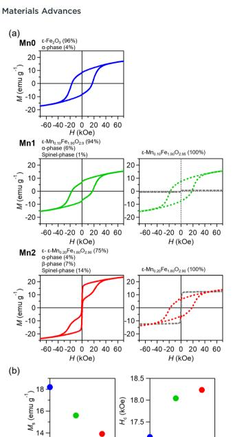
**Fig. 6** (a) Magnetisation *versus* external magnetic field curves at 300 K for (left) observed and (right) estimated curves. Coloured and grey lines represent the curve for the contributions of the  $\epsilon$ -Mn<sub>x</sub>Fe<sub>2-x</sub>O<sub>3-x/2</sub> and spinel-phase, respectively. (b)  $M_{\rm s}$  and  $H_{\rm c}$  *versus* x plot.
