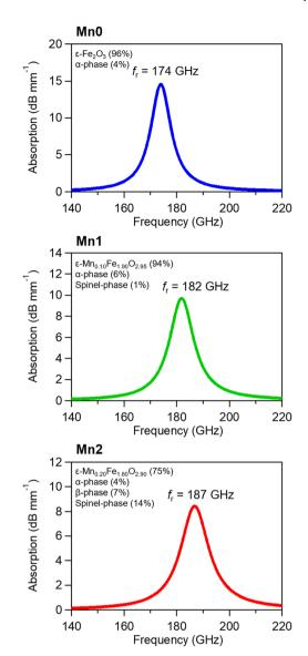
Fig. 7 Millimetre-wave absorption spectra of **Mn0**, **Mn1**, and **Mn2** normalized by the  $\epsilon$ -phase fraction and filling ratio. Fringe patterns from multiple reflections are removed.
