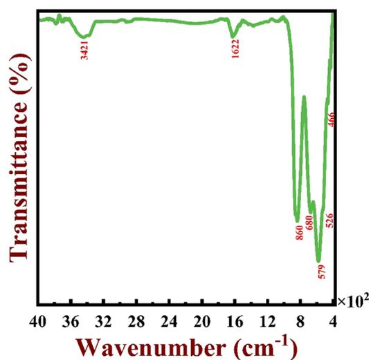
Fig. 4 FTIR spectrum of CoWO<sub>4</sub> nanostructures.
