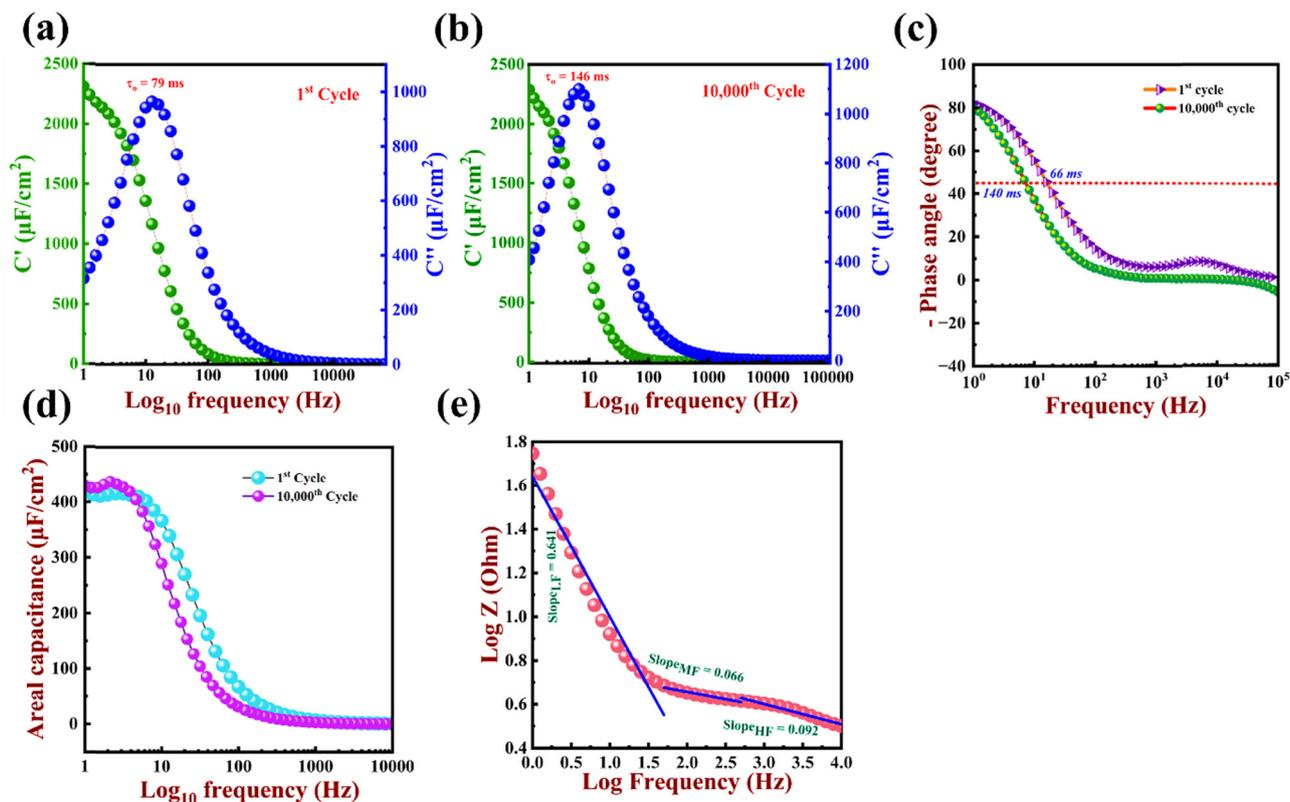
Fig. 11 (a)  $C'$  and  $C''$  vs. frequency of CoWO<sub>4</sub>//AC at the 1st cycle. (b)  $C'$  and  $C''$  vs. frequency of CoWO<sub>4</sub>//AC at the 10 000th cycle. (c) The phase angle log plot. (d) Areal capacitance vs. log frequency at the 1st and 10 000th cycle. (e) Impedance bode plot.
