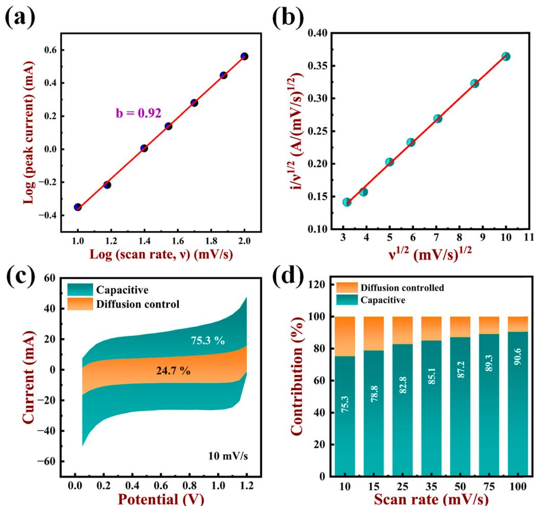
Fig. 12 (a)  $\log i$  vs.  $\log \nu$  curve to get  $b$  value (b)  $i/v^{1/2}$  vs.  $\nu^{1/2}$  curve at 1 V potential utilized to compute the values of  $k_1$  and  $k_2$ . (c) Differentiating surface capacitive current and diffusion controlled current for the CoWO<sub>4</sub> electrode at 10 mV s<sup>-1</sup>. (d) The ratio of capacitive contribution at varying scan rates from 10 mV s<sup>-1</sup> to 100 mV s<sup>-1</sup> for the CoWO<sub>4</sub> electrode.
