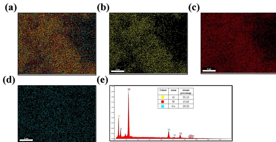
Fig. 7 (a) Simultaneous elemental mapping image, which confirmed the presence of (b) oxygen; (c) tungsten; (d) cobalt, and (e) the EDX spectrum of CoWO<sub>4</sub>.
