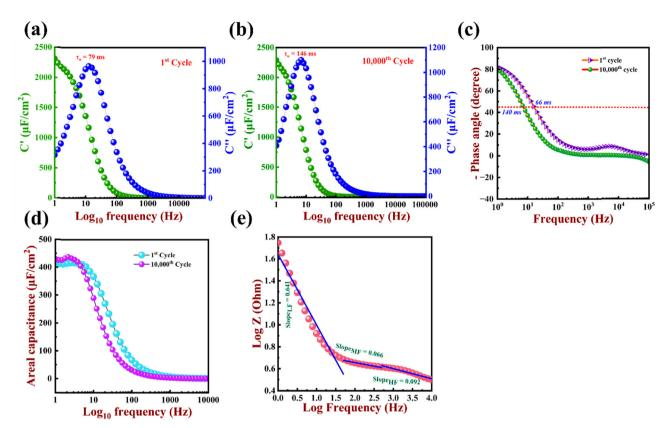
Fig. 11 (a) C' and C" vs. frequency of CoWO<sub>4</sub>||AC at the 1st cycle. (b) C' and C" vs. frequency of CoWO<sub>4</sub>||AC at the 10 000th cycle. (c) The phase angle bode plot. (d) Areal capacitance vs. log frequency at the 1st and 10 000th cycle. (e) Impedance bode plot.
