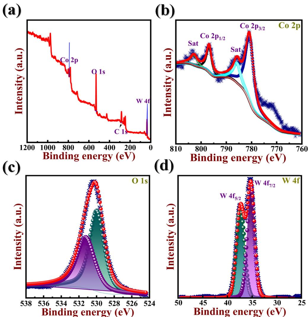
Fig. 8 (a) Comprehensive XPS survey scan, (b) Co 2p core level, (c) O 1s core level and (d) W 4f core level scan of the as-synthesized CoWO<sub>4</sub> powder.
