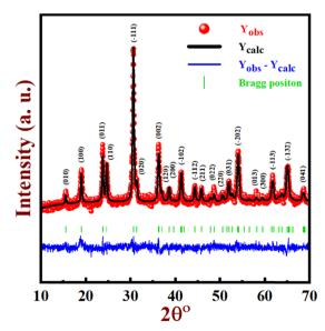
Fig. 1 Powder XRD pattern and Rietveld refinement of CoWO<sub>4</sub>.
