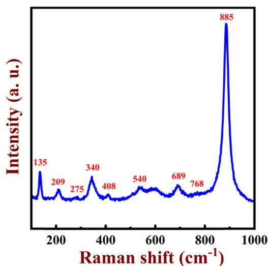
Fig. 3 Raman spectroscopy of CoWO<sub>4</sub> nanostructures.
