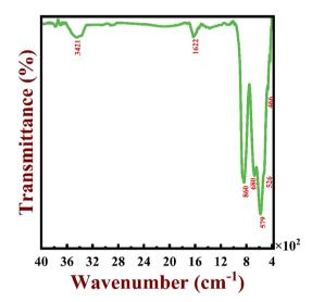
Fig. 4 FTIR spectrum of CoWO<sub>4</sub> nanostructures.
