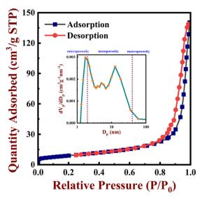
Fig. 5 The gas adsorption-desorption isotherm curve of CoWO<sub>4</sub> and inset shows the BJH plot for the porosity evolution of CoWO<sub>4</sub>.
