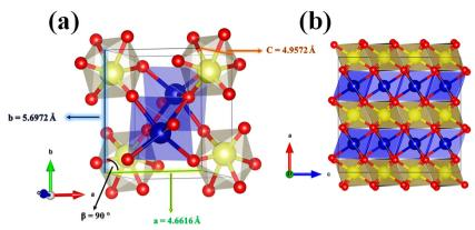
Fig. 2 (a) An illustration of  $CoWO_4$  showing the octahedral structure of  $CoO_6$  and  $WO_6$  as represented by the spheres of cobalt (blue), tungsten (yellow), and oxygen (red). (b) The  $CoWO_4$  unit cell is projected onto the (0 1 0) plane, revealing the alternate networks of the  $WO_6$  and  $CoO_6$  octahedron towards the [0 0 1] direction.
