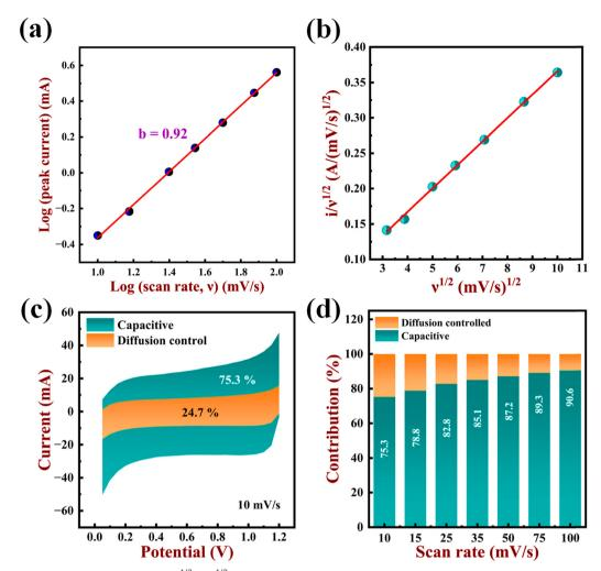
Fig. 12 (a)  $\log i$  vs.  $\log \nu$  curve to get b value (b)  $i/\nu^{1/2}$  vs.  $\nu^{1/2}$  curve at 1 V potential utilized to compute the values of  $k_1$  and  $k_2$ . (c) Differentiating surface capacitive current and diffusion controlled current for the CoWO<sub>4</sub> electrode at 10 mV s<sup>-1</sup>. (d) The ratio of capacitive contribution at varying scan rates from 10 mV s<sup>-1</sup> to 100 mV s<sup>-1</sup> for the CoWO<sub>4</sub> electrode.
