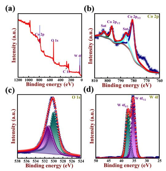
(a) Comprehensive XPS survey scan, (b) Co 2p core level, (c) O 1s core level and (d) W 4f core level scan of the as-synthesized CoWO<sub>4</sub> powder.
