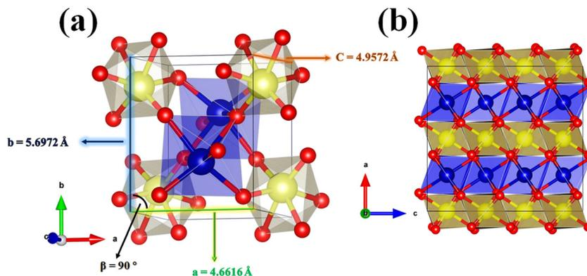
Fig. 2 (a) An illustration of CoWO<sub>4</sub> showing the octahedral structure of CoO<sub>6</sub> and WO<sub>6</sub> as represented by the spheres of cobalt (blue), tungsten (yellow), and oxygen (red). (b) The CoWO<sub>4</sub> unit cell is projected onto the (0 1 0) plane, revealing the alternate networks of the WO<sub>6</sub> and CoO<sub>6</sub> octahedron towards the [0 0 1] direction.
