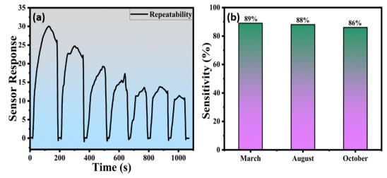
Fig. 8 (a) Repeatability of the sensor substrate  $Ba_{0.98}Sr_{0.02}Sn_{0.95}Mn_{0.05}O_3$  at room temperature ( $\sim 25$  °C) and a humidity of  $\sim 70\%$  for ethanol (100 ppm) and (b) the sensitivity of the Ba<sub>0.98</sub>Sr<sub>0.02</sub>Sn<sub>0.95</sub>Mn<sub>0.05</sub>O<sub>3</sub> sensor substrate probed in March, August and October (2024).
