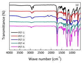
Fig. 3 FTIR spectra of (a) PET waste samples and (b) their ashes.
