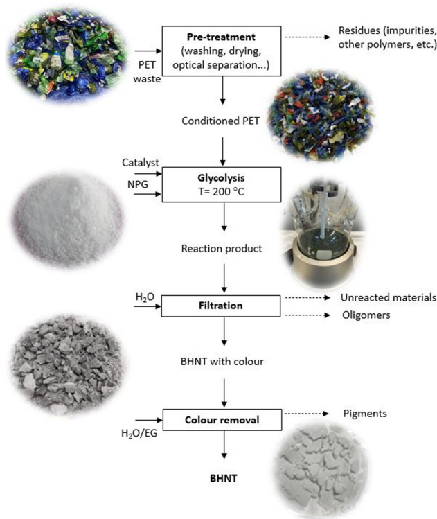
Fig. 2 The PET glycolysis reaction and product purification process.
