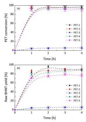
Fig. 5 Effect of the reaction time on (a) PET conversion and (b) raw BHNT yield.
