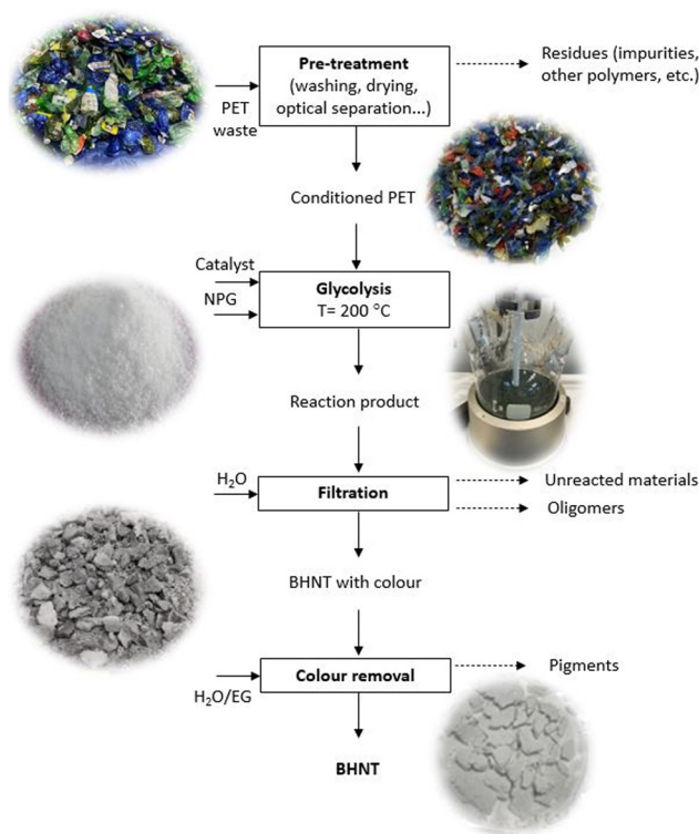
Fig. 2 The PET glycolysis reaction and product purification process.
