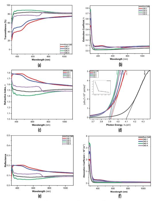
Fig. 6 Variations of the (a) optical transmittance, (b) extinction coefficient, (c) refractive index, (d) optical band gap with photon energy, (e) reflectance, and (f) absorption coefficient of the deposited thin films.
