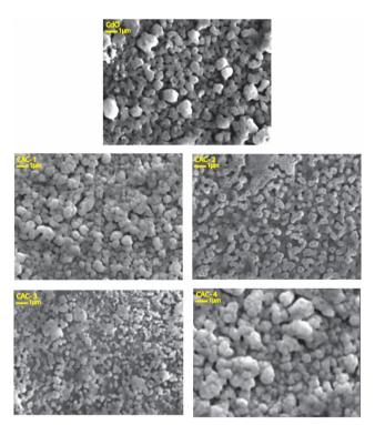
Fig. 4 Scanning electron microscopy images of the pure CdO and Ag-Co dual-doped CdO thin films
