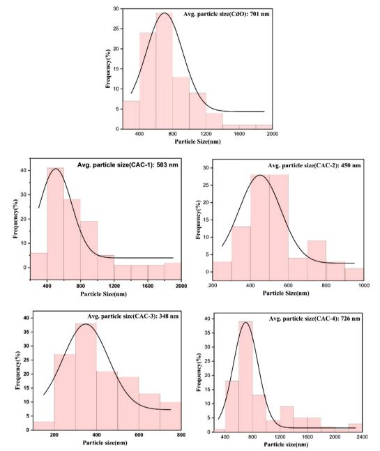
Fig. 5 Average particle sizes obtained from the histogram images of pure CdO and Ag-Co dual-doped CdO thin films.
