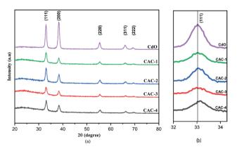
Fig. 2 (a) X-ray diffraction (XRD) patterns and (b) peak shifting (111) plane of the pure CdO and Ag-Co dual-doped CdO thin films.
