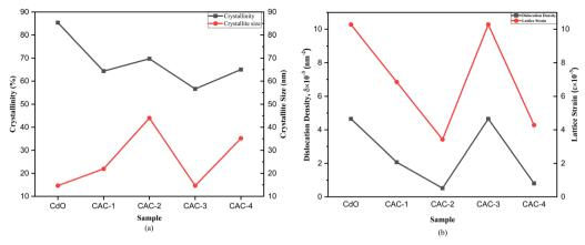
Fig. 3 Variation of the (a) crystallinity and crystallite size and (b) dislocation density and lattice strain of the pure CdO and Ag-Co dual-doped CdO thin films.
