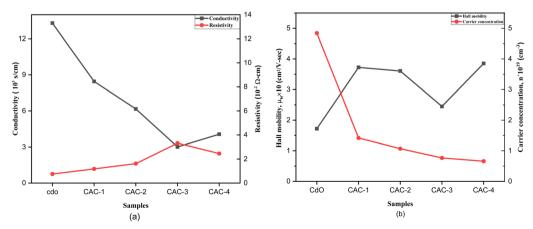
Fig. 7 Variations of the (a) resistivity and conductivity, and (b) Hall mobility ( $\mu_H$ ) and carrier concentrations (n) of the pure CdO and Ag-Co dual-doped CdO thin films.
