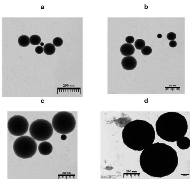
**Fig. 2** TEM images depict (a) Au/MIP1, (b) Au/MIP2, (c) Au/MIP3, and (d) Au/MIP4 at a 200 nm scale. These images showcase Au/MIP nanoparticles where the size of AuNPs was systematically varied to 5 nm, 20 nm, 50 nm, and 100 nm, respectively.
