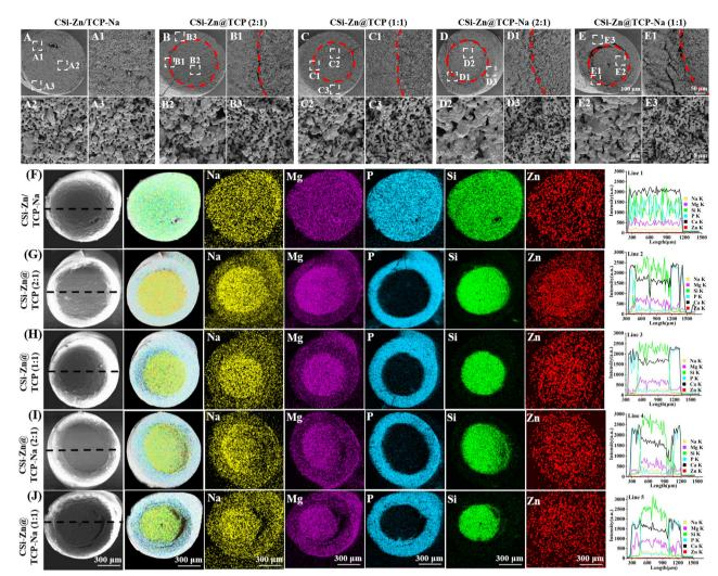
SEM microstructure and EDS analysis of bioceramic granules. (A)-(E) Microstructure of sintered core-shell bioceramic granules, with the red dashed lines indicating the boundary between the core and shell layers. (F)-(J) EDS mapping and line scan spectra of the cross-sections of bioceramic granules
