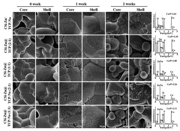
SEM observations and EDS analyses of bioceramic granules after immersion in SBF for different time periods.
