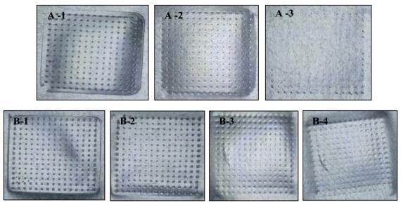
Fig. 5 Insertion depth on PF of the two-time intervals (A) 30 s-time intervals with the corresponding number of layers, (B) 1 min and the associated number of layers.
