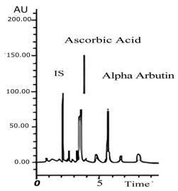
Fig. 8 LC-MS chromatogram of AA and ascorbic acid loaded MNs with IS (vitamin B6) at optimized chromatographic conditions. Column: Atlantis Premier BEH C18 AX Column (2.1 mm  $\times$  100 mm, particle size 1.7  $\mu$ m); mobile phase (A) 20 mM ammonium formate in water, mobile phase (B) 20 mM ammonium formate in methanol with gradient elution. The flow rate is 0.40 mL min $^{-1}$ .
