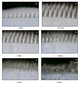
Fig. 7 Dissolution profile of the MN tips: 0, 0.5, 1, 2, 4 and 5 min.
