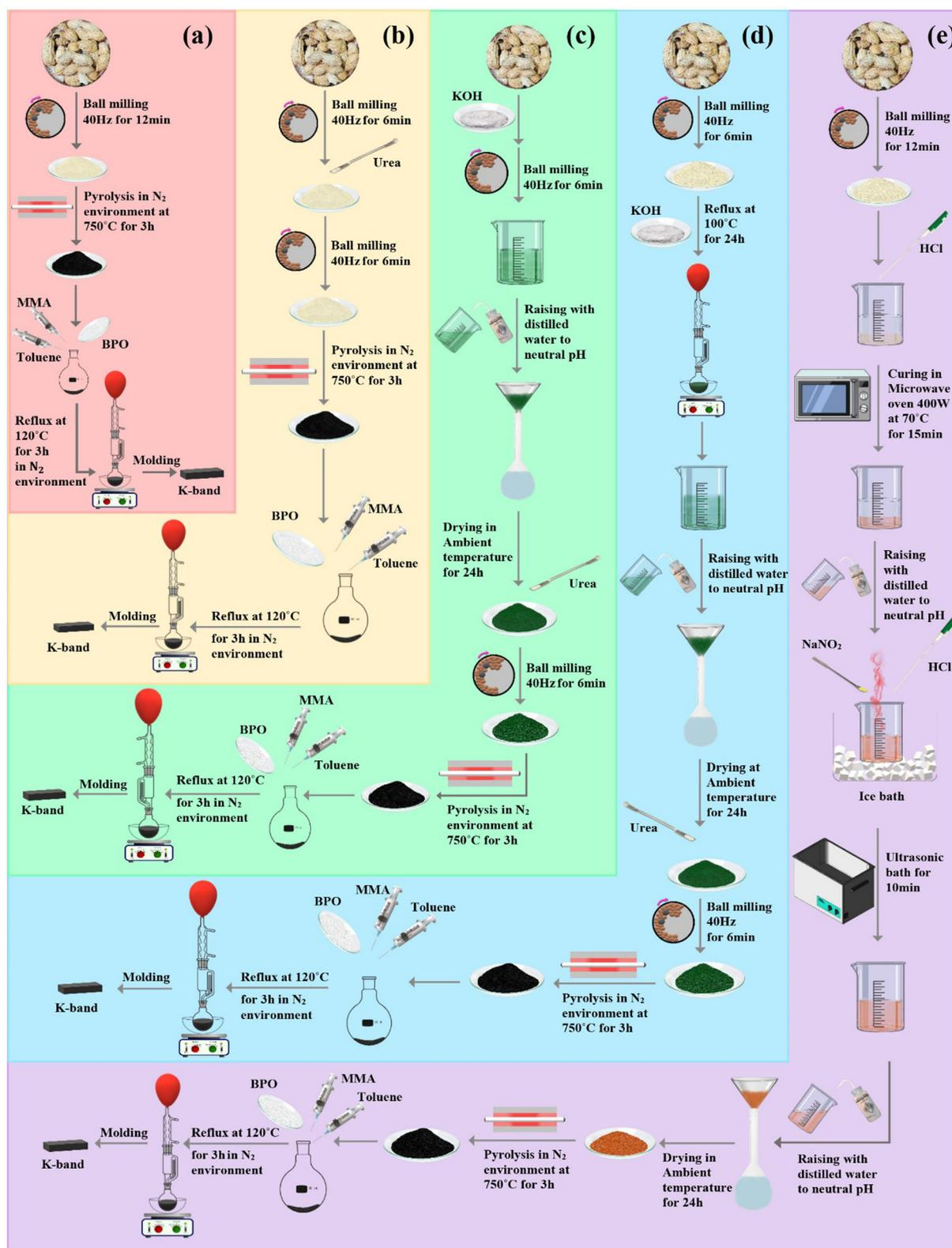
Fig. 1 Synthetic routes of C-PS (a), C-PS/U (b), C-PS/K/U-1 (c), C-PS/K/U-2 (d) and N-D-C-PS (e).
