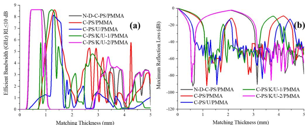
Fig. 7 Matching thickness associated with the highest result of efficient bandwidth (a) ( $RL \leq 10$  dB) and maximum RL (b) of PMMA-based composites.
