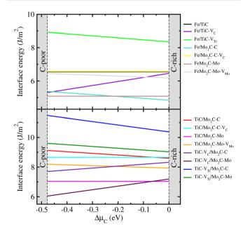
Fig. 6 Interface energy as a function of the chemical potential of carbon  $(\Delta\mu_{\rm C})$  varying from -0.48 eV to 0 for the interface systems.
