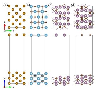
Fig. 2 Optimized structures of slab supercells for (a) Fe(100) (3  $\times$  2), (b) TiC(110) (2  $\times$  1), and (c) and (d) Mo<sub>2</sub>C(001) (2  $\times$  1) Mo- and C-terminated
