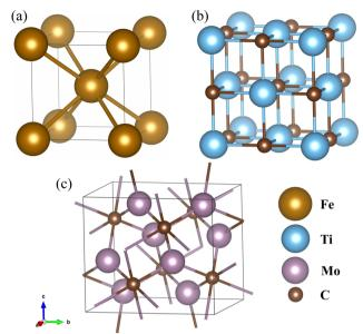
Fig. 1 Ball-and-stick view of unit cells for (a) iron in the bcc phase ( $\alpha$ -Fe), (b) titanium carbide (TiC) in the cubic phase, and (c) molybdenum hemicarbide in the orthorhombic phase (α-Mo<sub>2</sub>C)
