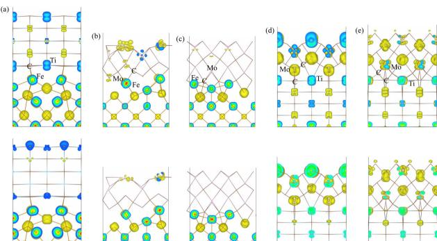
Fig. 8 Isosurface view of electron density calculated using the wave functions with energy levels from the Fermi level to +1 eV (top panel) and to -1 eV (bottom panel) in (a) Fe(100)/TiC(110), (b)  $Fe(100)/Mo_2C(001)-Mo$ , (c)  $Fe(100)/Mo_2C(001)-C$ , (d)  $TiC(110)/Mo_2C(001)-Mo$ , and (e)  $TiC(110)/Mo_2C(001)-C$ interfaces
