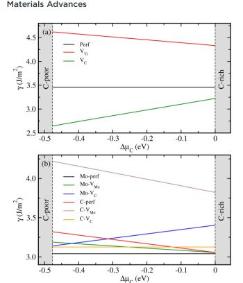
Fig. 3 Surface energy  $(\gamma)$  as functions of carbon chemical potential difference ( $\Delta\mu_{\rm C}$ ) for (a) TiC(110) surfaces and (b) Mo<sub>2</sub>C(001) Mo- and C-terminated surfaces, without and with a surface vacancy.
