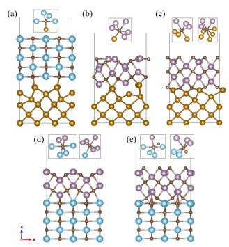
Fig. 4 Optimized structures of the slab supercells for interfaces of (a) Fe(100)/TiC(110), (b) and (c) Fe(100)/Mo<sub>2</sub>C(001) Mo- and C-terminations, and (d) and (e) TiC(110)/Mo<sub>2</sub>C(001) Mo- and C-terminations. The insets show all-metal or metal-carbon hybrid polyhedra centered at the C atom around the interface region.
