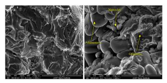
(a) SEM image of pure Al. (b) SEM image of the nanocomposite
