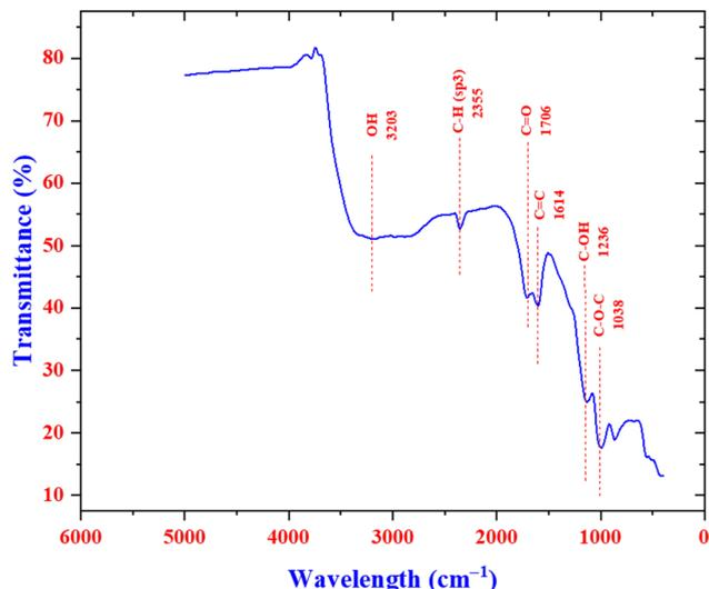
Fig. 5 FTIR spectra of graphene.
