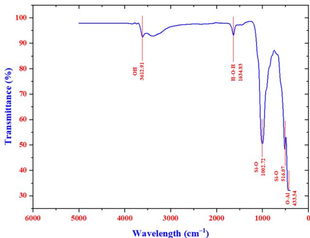
Fig. 6 FTIR spectra of bentonite nanoclay.
