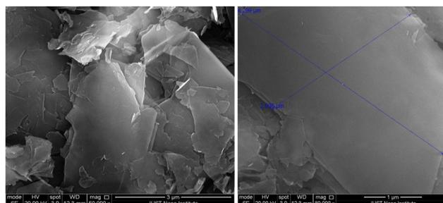
Fig. 4 SEM images of the prepared graphene sheets.
