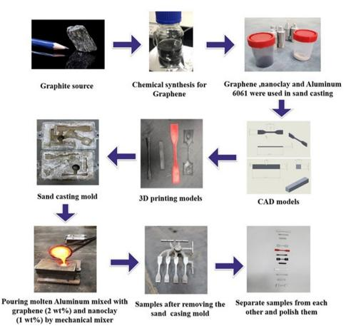
Fig. 3 The main steps for the preparation of the hybrid nanocomposite.
