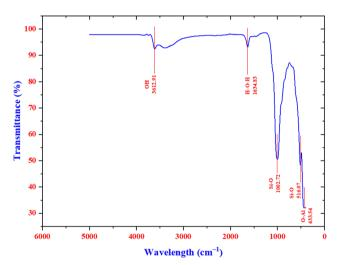
Fig. 6 FTIR spectra of bentonite nanoclay.
