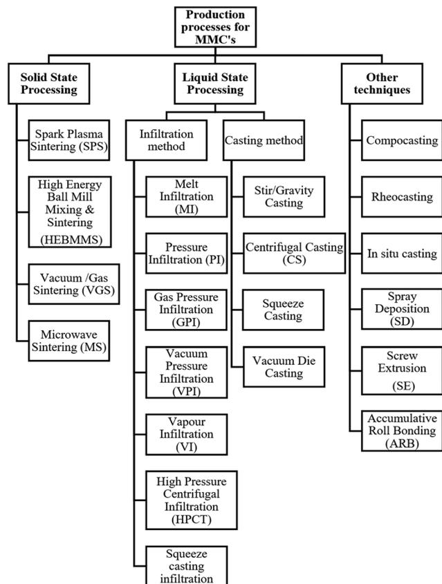
Fig. 1 Processing methods used for MMC fabrication.<sup>33</sup>
