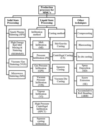
Fig. 1 Processing methods used for MMC fabrication.<sup>33</sup>
