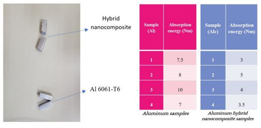
Fig. 9 Impact test results for the pure Al 6061-T6 matrix and the hybrid nanocomposite.
