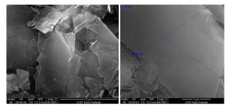
Fig. 4 SEM images of the prepared graphene sheets.
