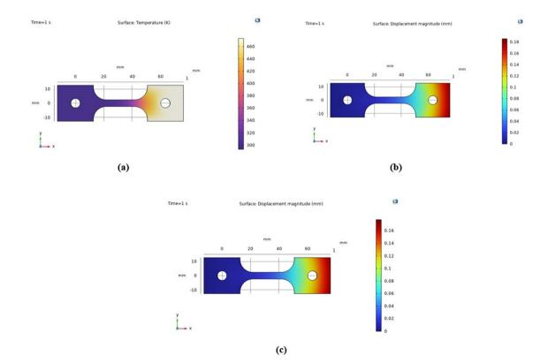
Fig. 13 Temperature distribution (a) and resultant total deformation in (b) the Al and (c) hybrid nanocomposite samples.
