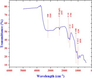
FTIR spectra of graphene.
