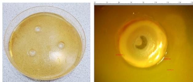
Fig. 7 Antimicrobial behavior of bentonite nanoclay with 2% concentration.
