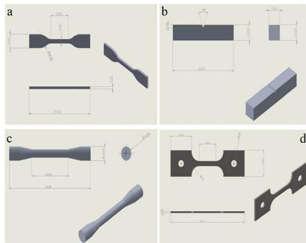
Fig. 2 3D design for the examination samples. (a) CAD model for tensile specimen. (b) CAD model for impact specimen. (c) CAD model for torsion specimen. (d) CAD model for creep specimen.
