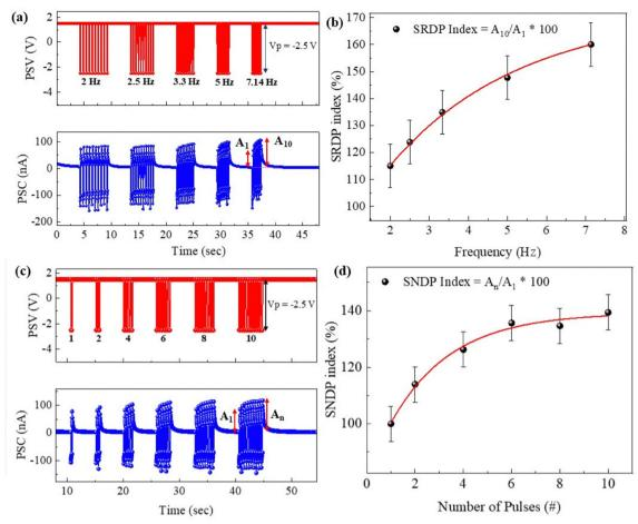
Fig. 6 Multiple pulse measurements performed using  $V_p = -2.5 \text{ V}$ . (a) SRDP measurements done by applying 10 consecutive voltage spikes of the same pulse width. (b) Dependence of SRDP index  $(A_{10}/A_1) \times 100$  on the frequency of application of pulses. (c) SNDP measurements performed by increasing the number of pulses (n = 1, 2, 4, ..., 10). (d) Dependence of SNDP index ( $A_n/A_1$ ) × 100 with pulse numbers.
