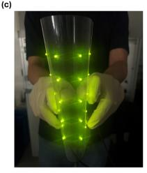
Fig. 4 (a) Circuit printed on a transparent PES substrate. (b) Operation of a flexible display with mounted LEDs without bending. (c) Operation of a flexible display with mounted LEDs under bending.
