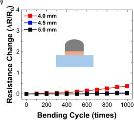
Fig. 2 Normalized change in resistance as a function of the 1000 cycles of the convex tensile bending tests conducted at radii of 4.0, 4.5, and 5.0 mm for (a) the SL and (b) DL electrodes.
