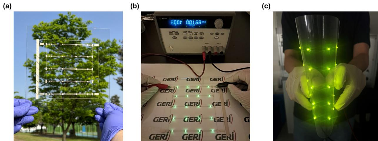
Fig. 4 (a) Circuit printed on a transparent PES substrate. (b) Operation of a flexible display with mounted LEDs without bending. (c) Operation of a flexible display with mounted LEDs under bending.
