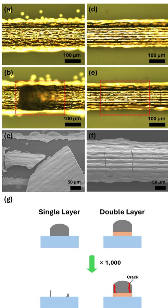
**Fig. 3** (a) and (d) OM images of SL and DL electrodes, respectively, before the tensile bending test. (b) and (e) OM images of SL and DL electrodes, respectively, after the tensile bending test. (c) and (f) SEM images of the regions marked with red-boxes in (b) and (e), respectively, providing detailed observations of the structures after the bending test. (g) Tensile bending test applied to both SL and DL electrodes.
