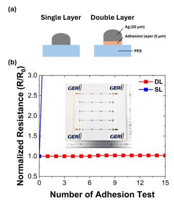
Fig. 1 (a) Electrode structures, exhibiting SL and DL electrodes. (b) Resistance measurement results indicating the change in resistance relative to the initial resistance as a function of the number of adhesion tests on the DL electrode. (Inset: image of a circuit printed on a PES substrate.)
