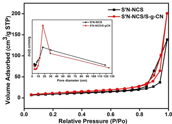
Fig. 4  $N_2$  adsorption–desorption isotherm of S'N-NCS and S'N-NCS/S-g-CN.
