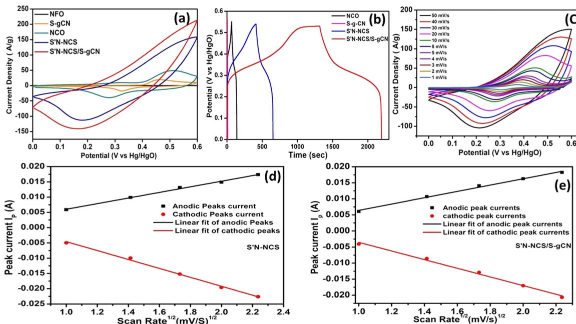
Fig. 5 (a) Comparative CV profile for NFO, NCO, S-g-CN, S'N-NCS and S'N-NCS/S-g-CN at  $100 \text{ mV s}^{-1}$ . (b) Comparative GCD profile of S'N-NCS/S-g-CN, S'N-NCS, NCO and S-g-CN at a current density of  $1 \text{ A g}^{-1}$  within the potential window of 0–0.53 V. (c) CV profile of S'N-NCS/S-g-CN at different scan rates varying from  $1 \text{ mV s}^{-1}$  to  $50 \text{ mV s}^{-1}$ . (d) and (e). Randles-Sevcik plot for S'N-NCS and S'N-NCS/S-g-CN.
