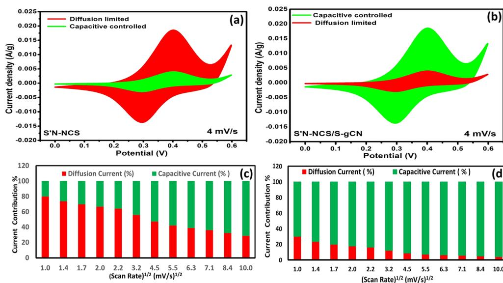
Fig. 7 Dunn's plot: (a) and (c) capacitive contribution for S'N-NCS and S'N-NCS/S-g-CN at  $4 \text{ mV s}^{-1}$ . Bar diagram of the percentage of capacitive and diffusion-controlled contributions for (b) and (d) S'N-NCS and S'N-NCS/S-g-CN at different scan rates.
