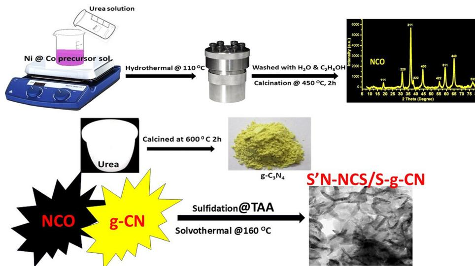
Scheme 1 Synthesis process of the S'N-NCS/S-g-CN nanocomposite.
