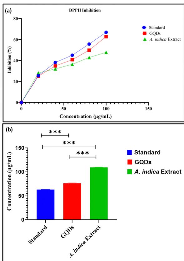
Fig. 5 Antioxidant potential of GQDs. (a) DPPH radical scavenging assay comparing the antioxidant activity of GQDs and neem extract, with GQDs showing enhanced activity. (b) Comparison of the IC<sub>50</sub> value of leaf extract and phyto-mediated GQDs with ascorbic acid. (Results presented as mean ± standard error. \*\*\* Significance level with control ( $p \leq 0.0001$ )).
