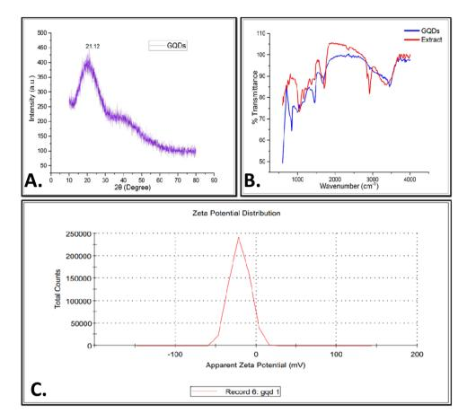
Fig. 2 Structural and chemical analysis of GQDs. (a) XRD pattern confirming the graphitic structure of GQDs with a prominent peak at  $21.1^{\circ}$ . (b) FTIR spectra revealing the functional groups of GQDs, including C=O, C-H, and O-H, indicating their successful functionalization. (c) Zeta potential analysis demonstrating the stability of GQDs with a negative charge of -22 mV, which is attributed to the presence of carboxyl and hydroxyl groups on the surface.
