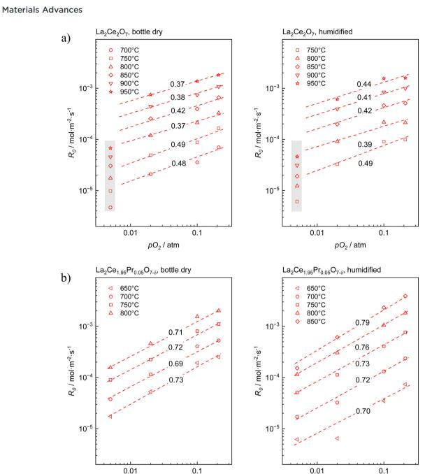
Fig. 3 Overall oxygen exchange rate,  $\Re_0$ , as a function of the oxygen partial pressure,  $p_{\mathcal{O}_2}$ , for (a)  $L_{a_2}Ce_2O_{7-\delta}$  and (b)  $L_{a_2}Ce_{195}Pr_{0.05}O_{7-\delta}$  with dry and wet carrier gases. The dashed lines represent least-squares fitting of the data according to  $\Re_0 \propto p_{\mathcal{O}_2}^m$  and the respective slopes, m, are included. Notably, all graphs exhibit the same ranges on the axes to facilitate comparison.
