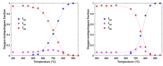
Fig. 2 Oxygen isotopologue fractions as a function of temperature for  $La_2Ce_{1.95}Pr_{0.05}O_{7-\delta}$  at  $p_{O_{\gamma}}=0.02$  atm in dry carrier gas (on the left) and wet carrier gas (on the right), respectively. In both cases, dry pulses were employed. The dotted lines represent the fits to the models (see ESI,† Section S1 and eqn (S17), (S22)–(S24)).
