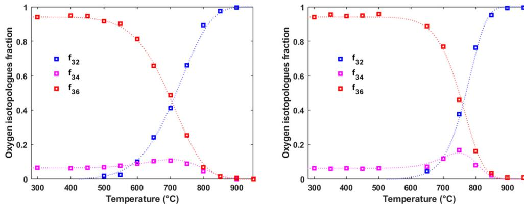
Fig. 2 Oxygen isotopologue fractions as a function of temperature for  $\text{La}_2\text{Ce}_{1.95}\text{Pr}_{0.05}\text{O}_{7-\delta}$  at  $p_{\text{O}_2} = 0.02$  atm in dry carrier gas (on the left) and wet carrier gas (on the right), respectively. In both cases, dry pulses were employed. The dotted lines represent the fits to the models (see ESI,† Section S1 and eqn (S17), (S22)–(S24)).
