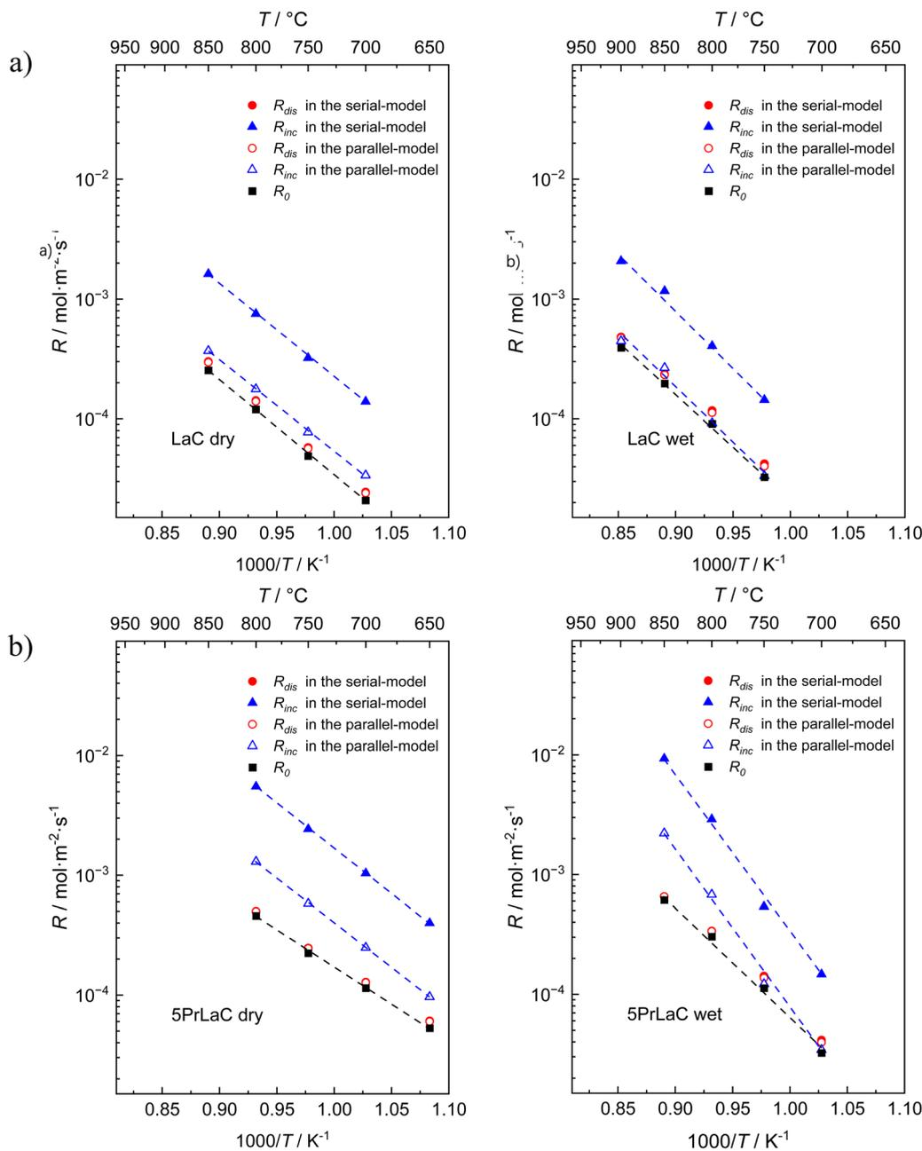
Fig. 7 Temperature dependence of the deconvoluted oxygen surface exchange rates in dry and wet carrier gases at  $p_{\text{O}_2} = 0.02$  atm, for (a)  $\text{La}_2\text{Ce}_2\text{O}_7$  and (b)  $\text{La}_2\text{Ce}_{1.95}\text{Pr}_{0.05}\text{O}_7$ . The entire dataset is presented in the Section S5 (ESI†).
