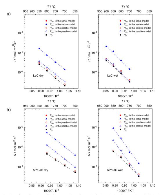
Fig. 7 Temperature dependence of the deconvoluted oxygen surface exchange rates in dry and wet carrier gases at  $p_{O_2} = 0.02$  atm, for (a) La<sub>2</sub>Ce<sub>2</sub>O<sub>7</sub> and (b)  $La_2Ce_{1.95}Pr_{0.05}O_7$ . The entire dataset is presented in the Section S5 (ESI†).
