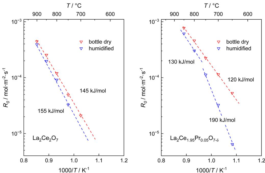
Fig. 5 Temperature dependence of the overall oxygen surface exchange rates of  $\text{La}_2\text{Ce}_2\text{O}_7$  and  $\text{La}_2\text{Ce}_{1.95}\text{Pr}_{0.05}\text{O}_{7-\delta}$  at  $p_{\text{O}_2} = 0.02$  atm in dry and wet carrier gases. In both cases, dry pulses were employed.
