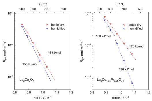
Fig. 5 Temperature dependence of the overall oxygen surface exchange rates of  $La_2Ce_2O_7$  and  $La_2Ce_{1.95}Pr_{0.05}O_{7-\delta}$  at  $p_{O_2}=0.02$  atm in dry and wet carrier gases. In both cases, dry pulses were employed.
