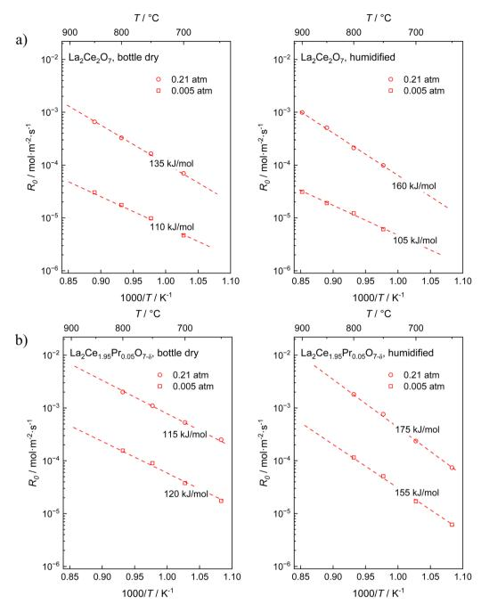
Fig. 4 Overall oxygen exchange rate,  $\Re_0$ , as a function of the inverse absolute temperature for the highest and lowest  $p_{O_2}$  for (a)  $La_2Ce_2O_{7-\delta}$  and (b)  $La_2Ce_{1.95}Pr_{0.05}O_{7-\delta}$  with dry and wet carrier gases. The dashed lines represent least-squares fitting of the data according to Arrhenius behavior, including the apparent activation energies. All graphs exhibit the same ranges on the axes to facilitate comparison.
