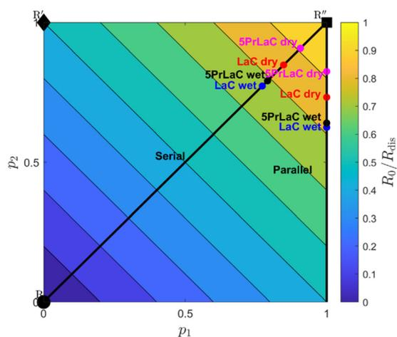
Fig. 6 Contour plot of the ratio of the overall oxygen exchange rate (hetero exchange rate) to the dissociative adsorption rate at 750 °C and 0.02 atm of  $\text{O}_2$ .  $p_1$  and  $p_2$  are the independent probabilities of each oxygen atom in a dissociated oxygen molecule being incorporated into the oxide. Further derivation and interpretation of the contour plot can be found in the ESI,<sup>†</sup> 72,74,75
