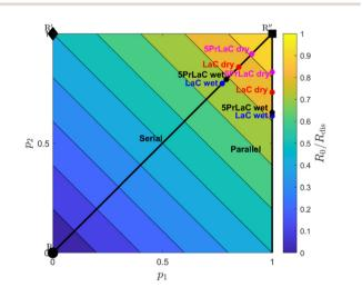
Fig. 6 Contour plot of the ratio of the overall oxygen exchange rate (hetero exchange rate) to the dissociative adsorption rate at 750 °C and 0.02 atm of O<sub>2</sub>.  $p_1$  and  $p_2$  are the independent probabilities of each oxygen atom in a dissociated oxygen molecule being incorporated into the oxide. Further derivation and interpretation of the contour plot can be found in the ESI.†  $^{72,74,75}\,$
