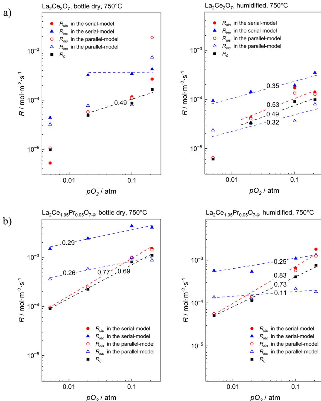
Fig. 8 Oxygen partial pressure dependence of the deconvoluted oxygen surface exchange rates in dry and wet carrier gases for (a)  $\text{La}_2\text{Ce}_2\text{O}_7$  and (b)  $\text{La}_2\text{Ce}_{1.95}\text{Pr}_{0.05}\text{O}_{7-\delta}$ . The entire dataset is presented in the Section S5 (ESI†).
