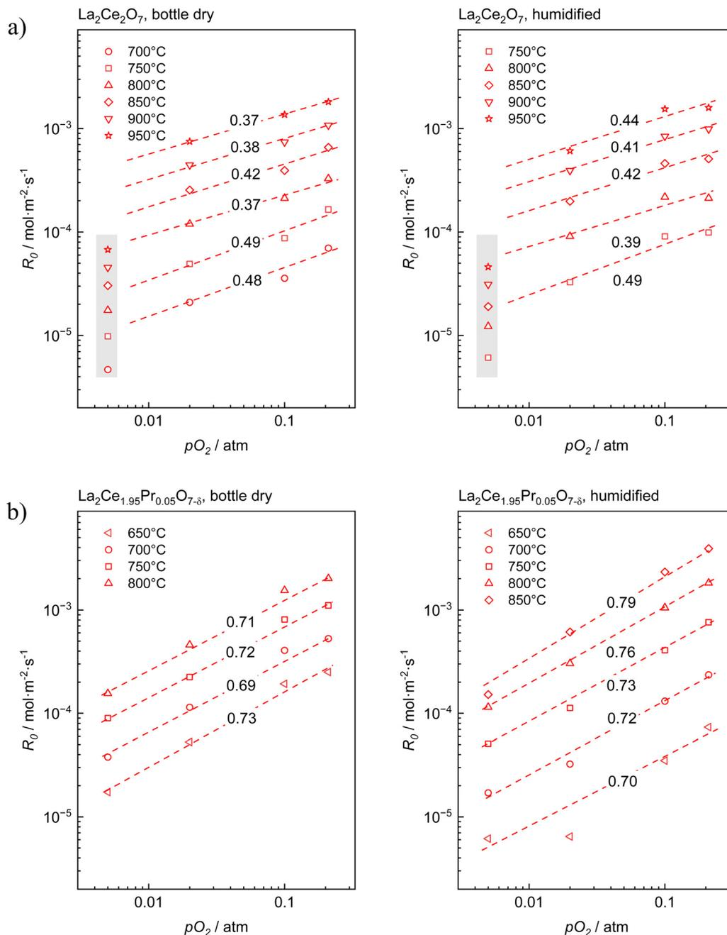
**Fig. 3** Overall oxygen exchange rate,  $R_0$ , as a function of the oxygen partial pressure,  $p_{O_2}$ , for (a)  $La_2Ce_2O_{7-\delta}$  and (b)  $La_2Ce_{1.95}Pr_{0.05}O_{7-\delta}$  with dry and wet carrier gases. The dashed lines represent least-squares fitting of the data according to  $R_0 \propto p_{O_2}^m$  and the respective slopes,  $m$ , are included. Notably, all graphs exhibit the same ranges on the axes to facilitate comparison.
