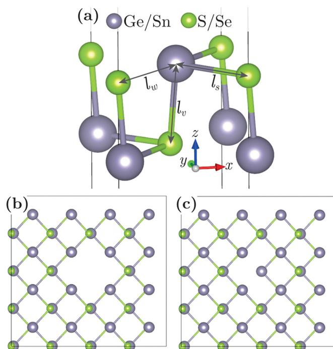
Fig. 1 (a) Crystal structure of the monolayer group IV monochalcogenides GeS, GeSe, SnS, and SnSe, where  $l_v$ ,  $l_s$ , and  $l_w$  represent the bond lengths of the vertical, strong, and weak bonds, respectively. Top view of a  $4 \times 4$  supercell of SnSe with (b) a pair of Sn and Se atoms removed (SnSe-p4) and (c) a single Se atom removed (SnSe-s4).
