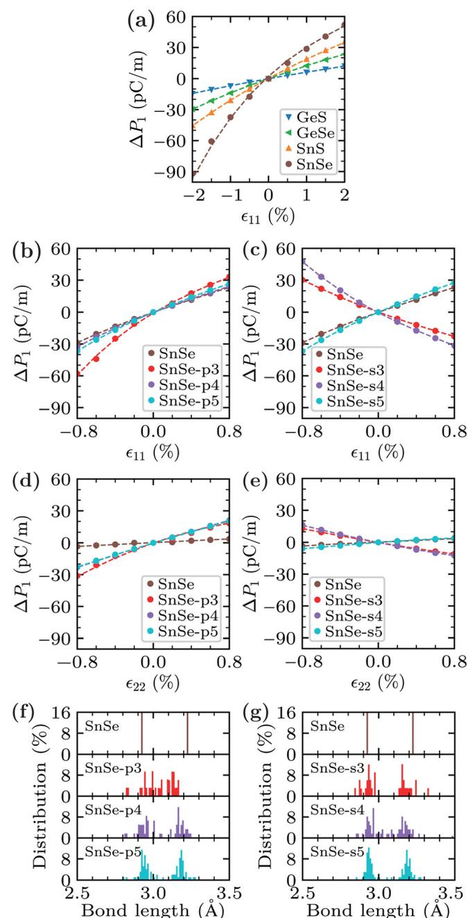
Fig. 3 Normalized polarization  $\Delta P_1 = P_1(\epsilon_{jk}) - P_1(0)$  under strain in (a) pristine monolayer GeS, GeSe, SnS, and SnSe as well as in monolayer SnSe with (b) and (d) Sn–Se and (c) and (e) Se vacancies. (f) and (g) Histograms of the intralayer bond lengths ( $l_s$  and  $l_w$ ).
