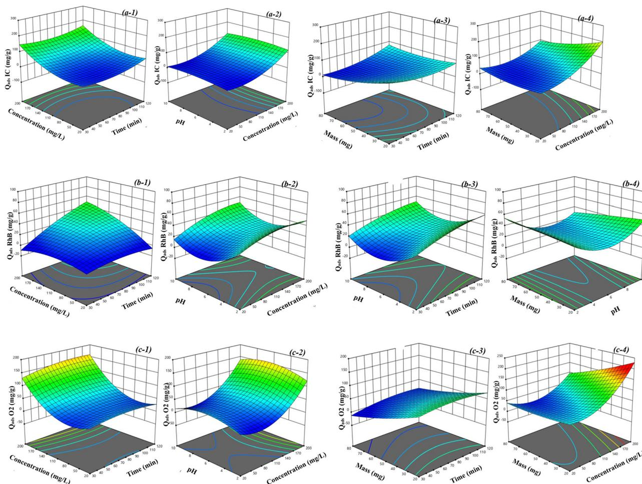
Fig. 5 3D response surface plots of the central composite design showing the effect of time (min), concentration of dye solution ( $\text{mg L}^{-1}$ ), pH and mass (mg) on the adsorption of indigo carmine (IC) (a-1)–(a-4), rhodamine B (RhB) (b-1)–(b-4) and orange 2 (O2) (c-1)–(c-4), respectively.
