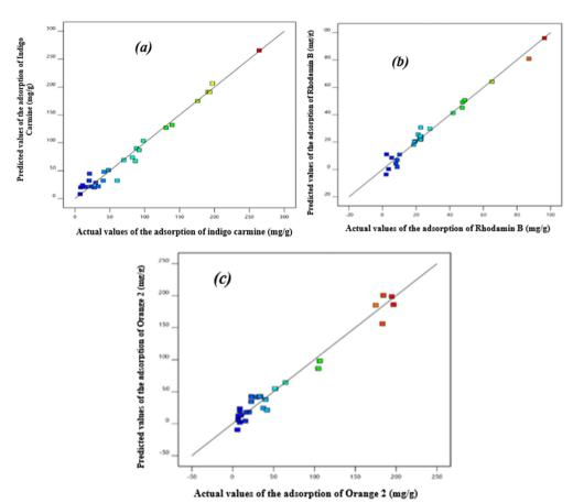
Fig. 4 Predicted values vs. observed values of the adsorption of indigo carmine (a), rhodamine B (b) and orange 2 (c) on NH<sub>2</sub>-UiO-66.
