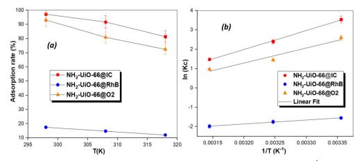
Fig. 8 Impact of the temperature on the adsorption of dyes using NH<sub>2</sub>-UiO-66 (a) and a plot of  $\ln(K_c)$  versus 1/T (K<sup>-1</sup>) (b).
