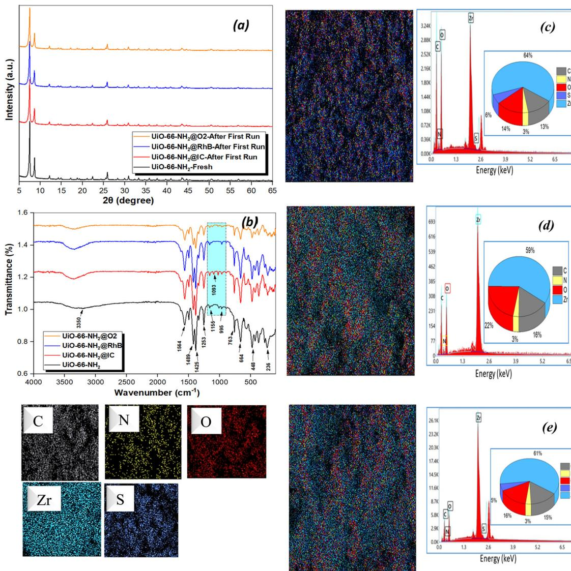
Fig. 10 PXR pattern (a) and FT-IR spectra (b) of fresh NH<sub>2</sub>-UiO-66 and after adsorption of dyes, EDX/EDX-mapping of NH<sub>2</sub>-UiO-66 after indigo carmine (IC) (c), rhodamine B (d) (RhB) and orange 2 (O2) (e) adsorption.
