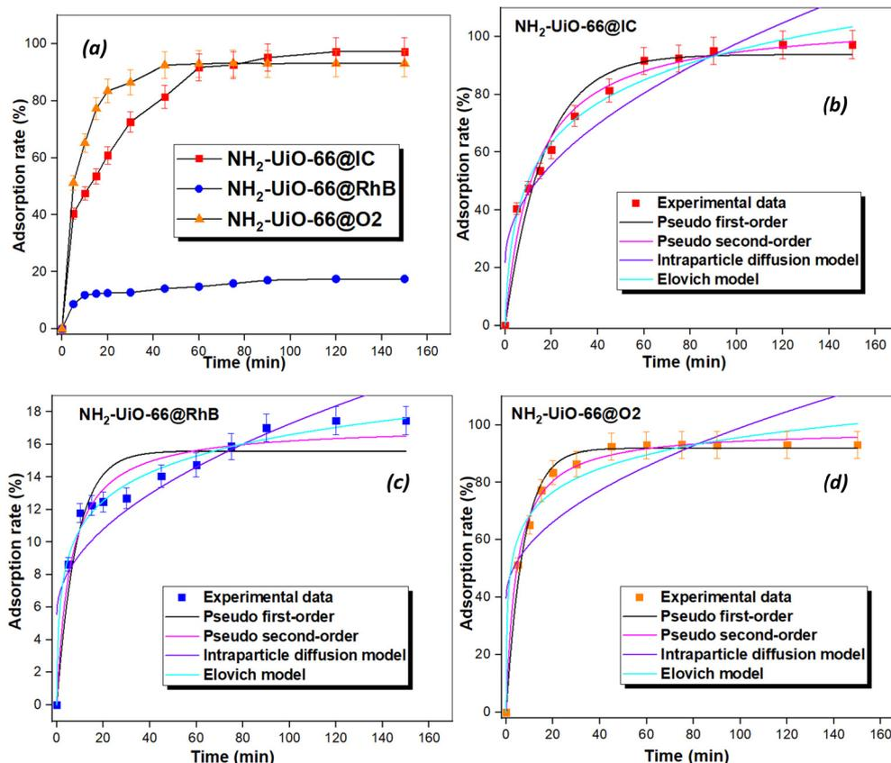
Fig. 7 Impact of stirring time on the adsorption of dyes using  $\text{NH}_2\text{-UiO-66}$  (a), non-linear experimental data fitted with pseudo first-order, pseudo second-order, intraparticle diffusion and the Elovich model for indigo carmine (b), rhodamine B (c) and orange 2 (d).
