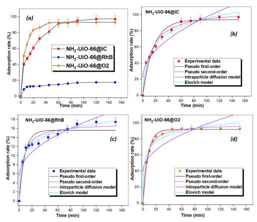
Fig. 7 Impact of stirring time on the adsorption of dyes using NH<sub>2</sub>-UiO-66 (a), non-linear experimental data fitted with pseudo first-order, pseudo second-order, intraparticle diffusion and the Elovich model for indigo carmine (b), rhodamine B (c) and orange 2 (d).
