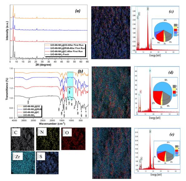
Fig. 10 PXRD pattern (a) and FT-IR spectra (b) of fresh NH2-UiO-66 and after adsorption of dyes, EDX/EDX-mapping of NH2-UiO-66 after indigo carmine (IC) (c), rhodamine B (d) (RhB) and orange 2 (O2) (e) adsorption.
