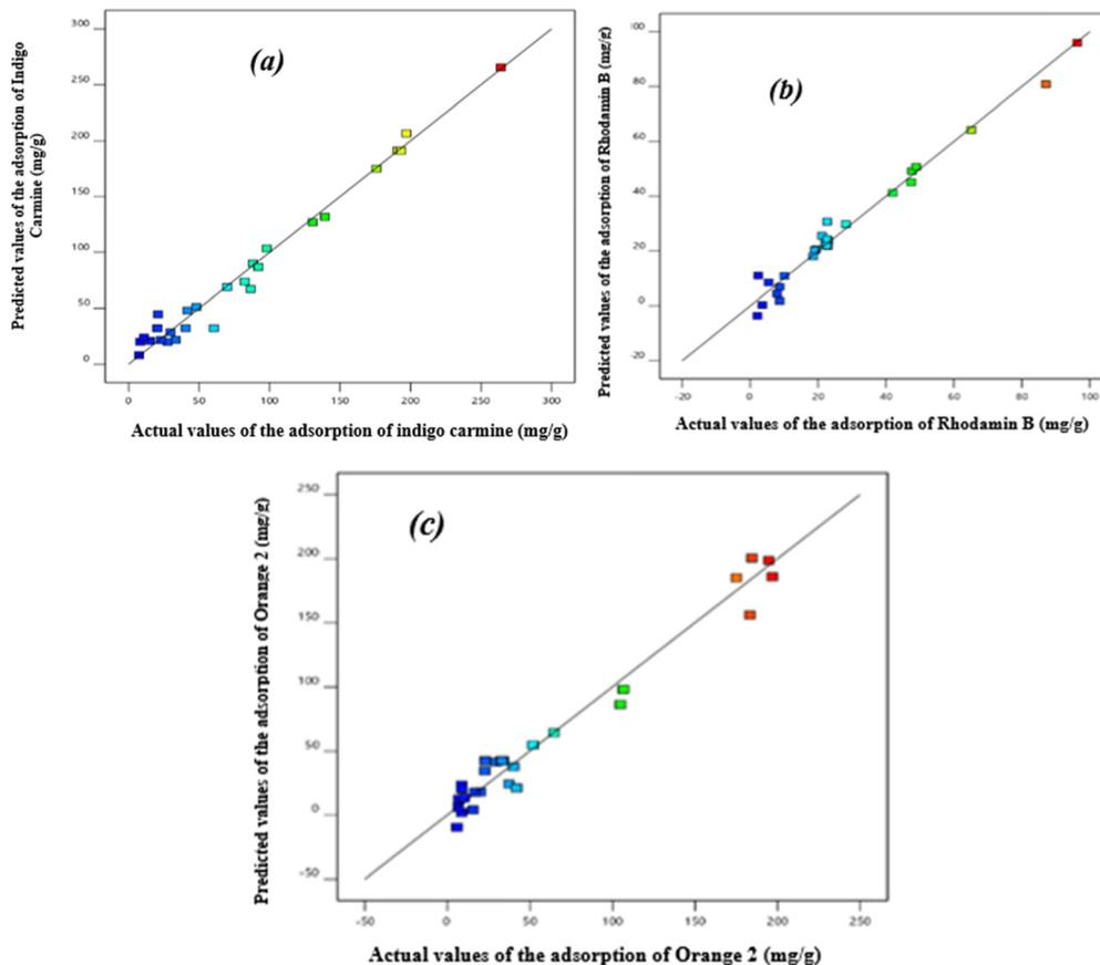
Fig. 4 Predicted values vs. observed values of the adsorption of indigo carmine (a), rhodamine B (b) and orange 2 (c) on  $\text{NH}_2\text{-UiO-66}$ .
