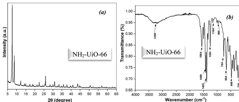
Fig. 1 PXRD pattern (a) and FTIR spectra (b) of NH<sub>2</sub>-UiO-66.
