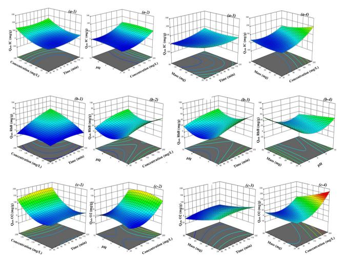
Fig. 5 3D response surface plots of the central composite design showing the effect of time (min), concentration of dye solution (mg  $L^{-1}$ ), pH and mass (mg) on the adsorption of indigo carmine (IC) (a-1)-(a-4), rhodamine B (RhB) (b-1)-(b-4) and orange 2 (O2) (c-1)-(c-4), respectively.
