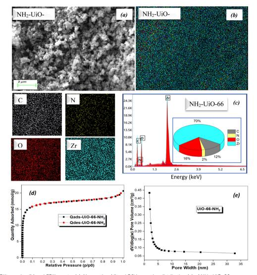
Fig. 2 SEM (a), EDX mapping (b) and EDX spectra (c), N<sub>2</sub> sorption (d) and BJH pore size distribution (e) of NH<sub>2</sub>-UiO-66.
