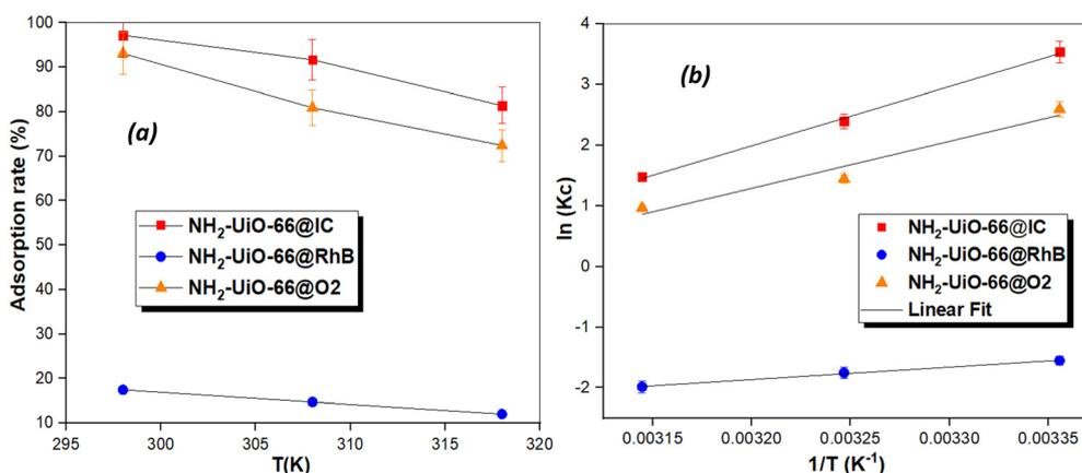
Fig. 8 Impact of the temperature on the adsorption of dyes using  $\text{NH}_2\text{-UiO-66}$  (a) and a plot of  $\ln(K_c)$  versus  $1/T$  ( $\text{K}^{-1}$ ) (b).
