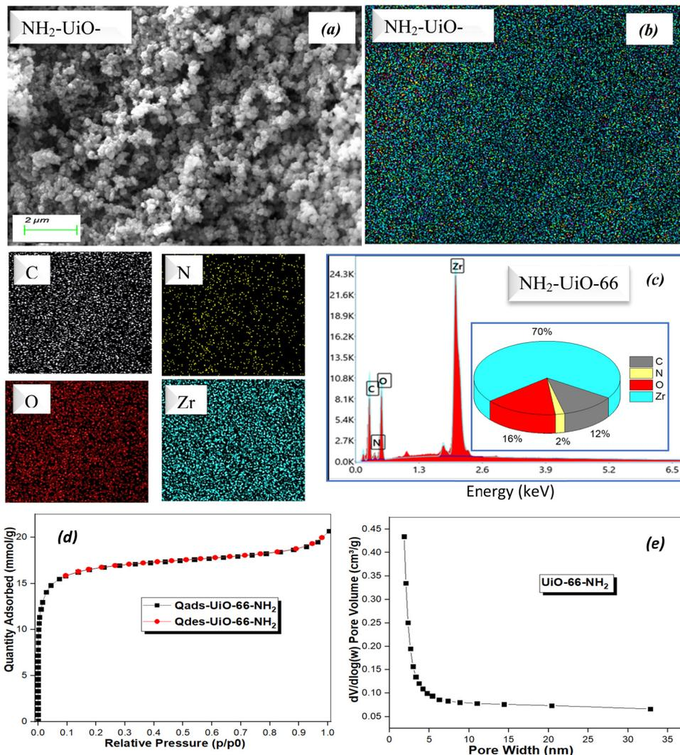
Fig. 2 SEM (a), EDX mapping (b) and EDX spectra (c), N<sub>2</sub> sorption (d) and BJH pore size distribution (e) of NH<sub>2</sub>-UiO-66.
