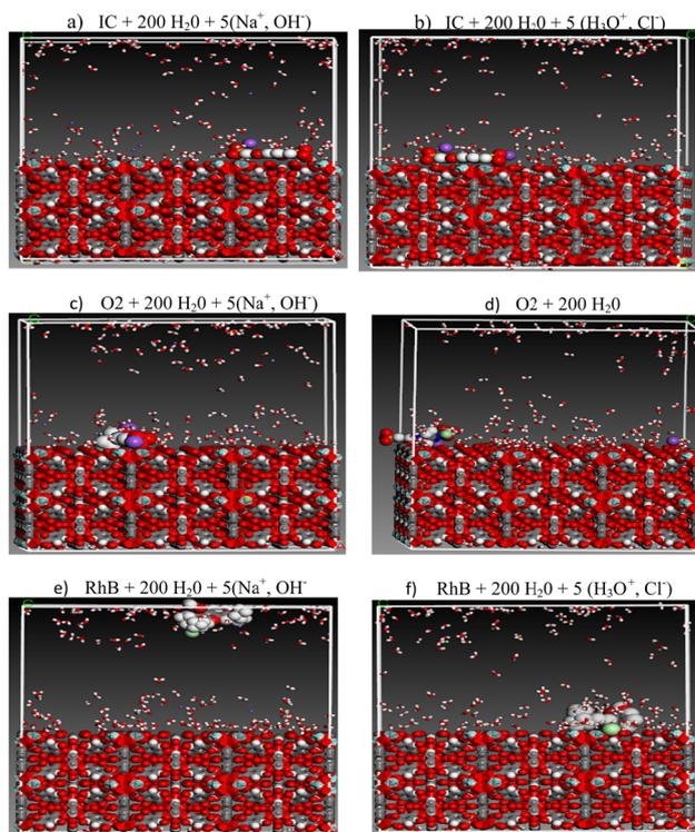
Fig. 12 Front views of the most stable low-energy configuration for the adsorption of IC (a and b), O2 (c and d) and RhB (e and f) dyes with  $\text{NH}_2$ -UiO-66 at 298 K in acidic, basic and neutral medium.
