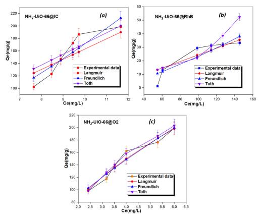
Fig. 6 Impact of concentration on the adsorption of dye using NH<sub>2</sub>-UiO-66 and non-linear experimental data fitted with Langmuir, Freundlich and Toth models for indigo carmine (a), rhodamine B (b) and orange 2 (c).
