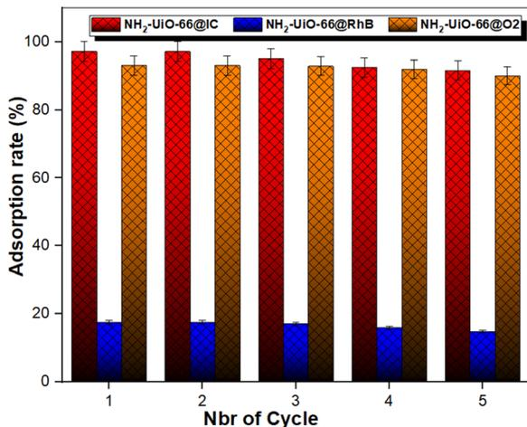
Fig. 9 Performance of NH<sub>2</sub>-UiO-66 for five consecutive cycles of indigo carmine (IC), rhodamine B (RhB) and orange 2 (O2) adsorption.
