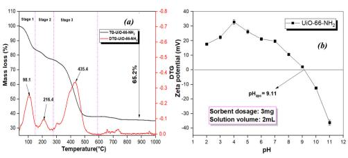
Fig. 3 TGA/DTG spectra (a) and zeta potential (b) of NH<sub>2</sub>-UiO-66.
