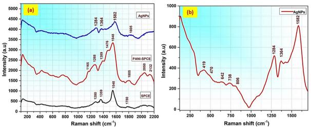
Raman spectra for the modified SPE: (a) comparison of the modified surface of the SPE and (b) Raman spectra of AgNPs.
