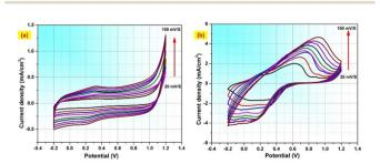
CV analysis of 4.0 mM lactic acid in PBS solution at different scan rates: (a) Ag-SPE and (b) Ag-PANI-SPE
