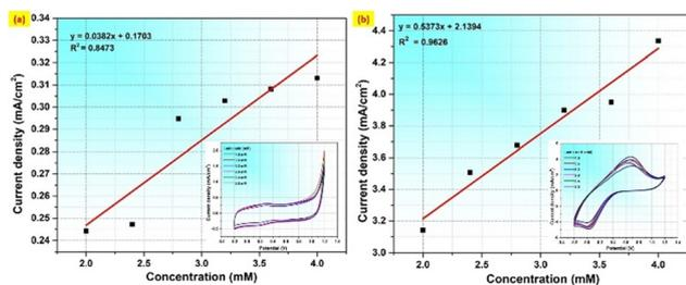
Fig. 11 Linearity curve with an increase in concentration: (a) Ag-functionalized SPE and (b) PANI/Ag functionalized SPE, for  $4.0 \text{ mM}$  lactic acid in PBS solution at  $100 \text{ mV s}^{-1}$  for the potential range of  $-0.2$  to  $1.2 \text{ V}$ .
