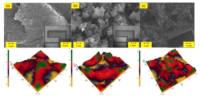
Fig. 4 FESEM images of the (a) bare, (b) PANI, and (c) Aq-PANI SPE surfaces, and an exploded view with an AFM micrograph.
