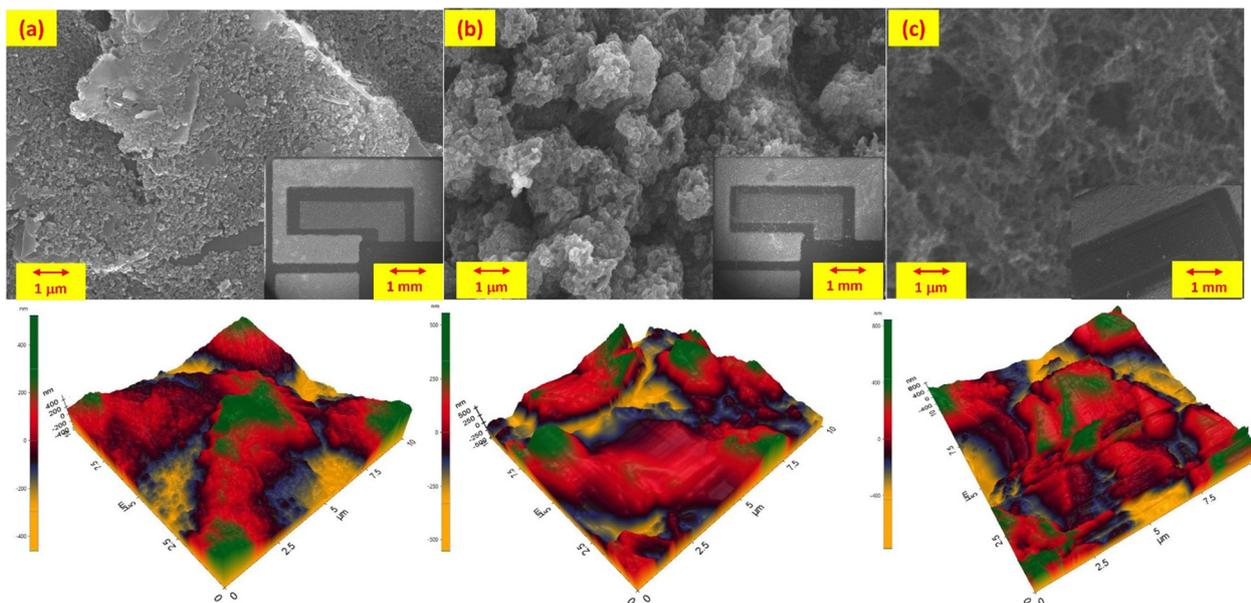
Fig. 4 FESEM images of the (a) bare, (b) PANI, and (c) Ag-PANI SPE surfaces, and an exploded view with an AFM micrograph.
