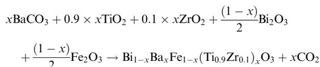
$\text{BaCO}_3$ ,  $\text{TiO}_2$ ,  $\text{ZrO}_2$ ,  $\text{Bi}_2\text{O}_3$ , and  $\text{Fe}_2\text{O}_3$  were used as starting reagents. These powders were accurately weighed in stoichiometric ratios and mixed thoroughly in an agate mortar for 1 hour.
