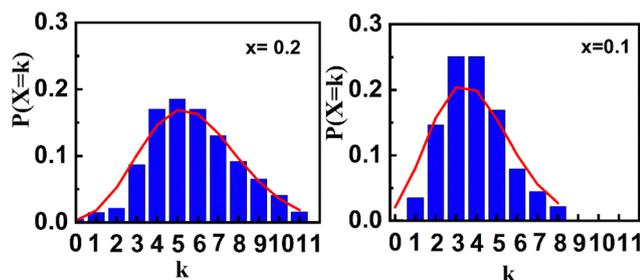
Fig. 9 Plots of the Poisson distribution expressing the probability that a  $\text{Fe}^{3+}$  site is surrounded by  $k$  nearest neighbors in  $\text{Ti}^{4+}$  and  $\text{Zr}^{4+}$  for both compositions,  $x = 0.1$  and  $x = 0.2$ . The blue bars represent the frequency histogram and the red curve corresponds to the Poisson distribution.
