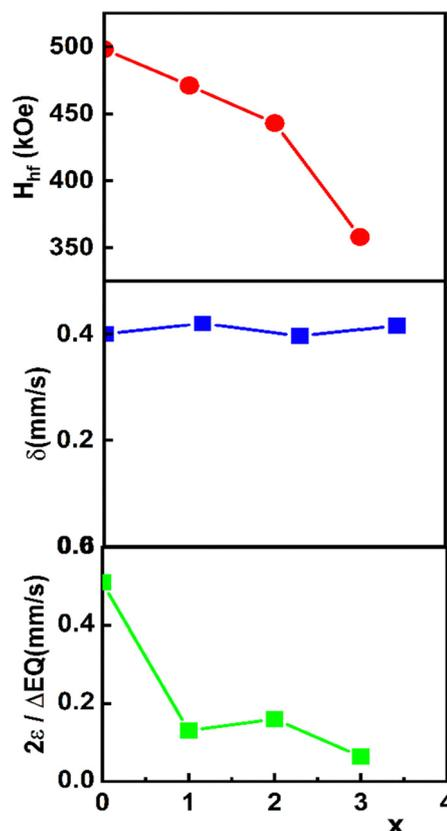
Fig. 10 Substitution rate dependence of mean hyperfine parameters values.  $H_{hf}$ : hyperfine field,  $\delta$ : isomer shift,  $\Delta E_Q/2\varepsilon$ : quadrupole splitting/shift.
