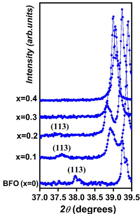
Fig. 3 Evolution of the superlattice reflection (113) for  $x = 0, 0.1, 0.2, 0.3$  and  $x = 0.4$ .
