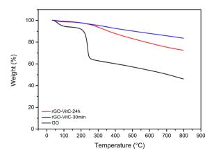
Fig. 1 TGA profiles of GO, rGO-VitC-30min and rGO-VitC-24h.
