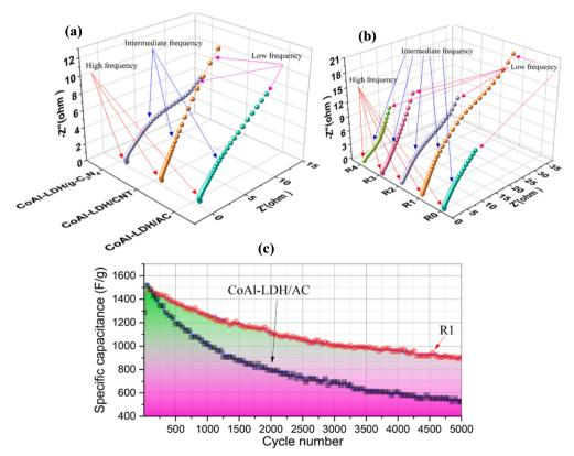
Fig. 12 (a) EIS graph of three electrodes. (b) EIS of the CoAl LDH/AC composite in different solvents. (c) Cycling stability of CoAl LDH/AC. Reproduced with permission from ref. 2.
