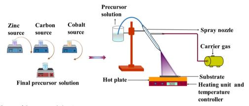
Fig. 1 Schematic diagram of the spray pyrolysis setup
