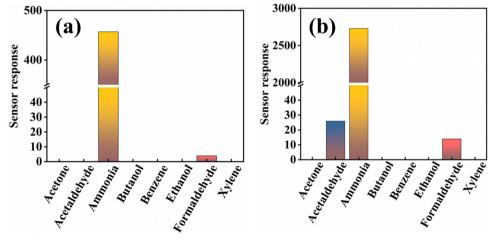
Fig. 11 Sensor responsiveness of the (a) CxZnO and (b) CxCoxZnO thin films towards various VOCs of 50 ppm at 300 K.
