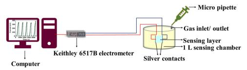
Fig. 2 Schematic representation of the sensing setup.
