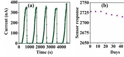
Fig. 13 (a) Repeatability study of the CxCoxZnO thin film and (b) stability study of the CxCoxZnO thin film for 50 ppm of ammonia.
