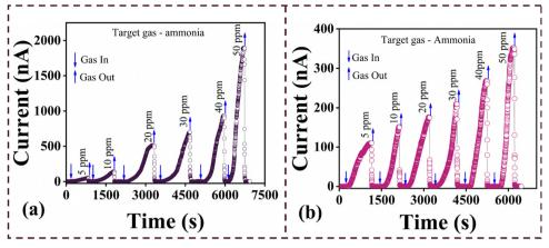
Transient response curve of the (a) CxZnO and (b) CxCoxZnO thin films towards different concentrations of ammonia
